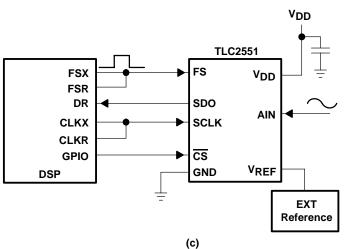
Figure 21. Typical TLC2551 Interface to a TMS320 DSP
