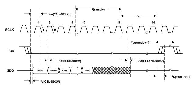
Figure 7. TLC2551 Critical Timing (Control via  $\overline{CS}$  only, FS = 1)
