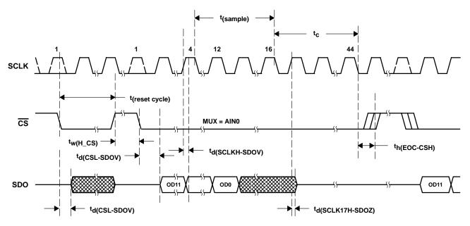
Figure 8. TLC2552 Reset Cycle Critical Timing
