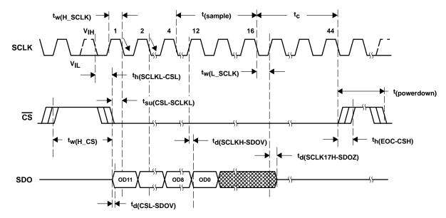
Figure 9. TLC2552 and TLC2555 Conversion Cycle Critical Timing
