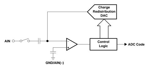
Figure 1. Simplified SAR Circuit
