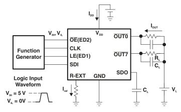
Figure 6. Test Circuit for Switching Characteristics
