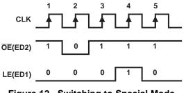
Figure 12. Switching to Special Mode
