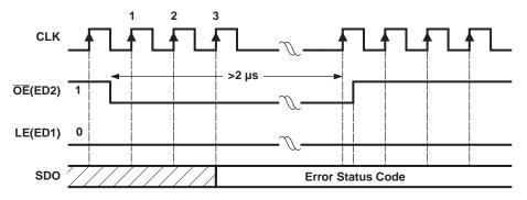
Figure 14. Reading Error Status Code
