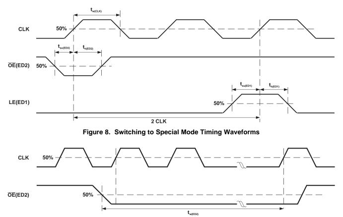
Figure 9. Reading Error Status Code Timing Waveforms
