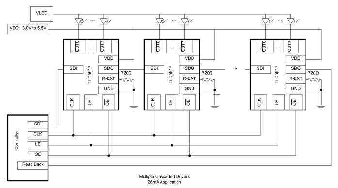
Figure 20. Cascading Implementation of TLC591x Device
