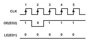
Figure 15. Switching to Normal Mode
