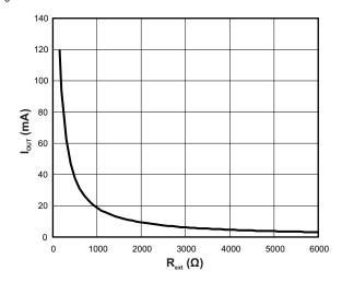
Figure 19. Default Relationship Curve Between  $I_{OUT,target}$  and  $R_{ext}$  After Power Up
