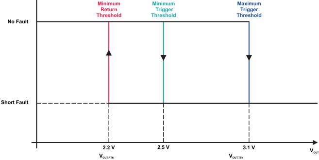
Figure 10. Short-Circuit Detection Principle
