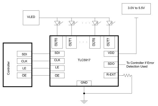
Figure 22. Single Implementation of TLC591x Device
