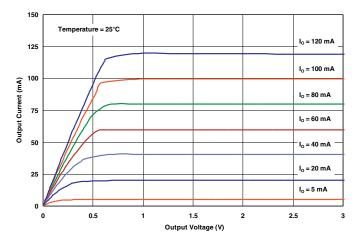
Figure 23. Output Current vs Output Voltage
