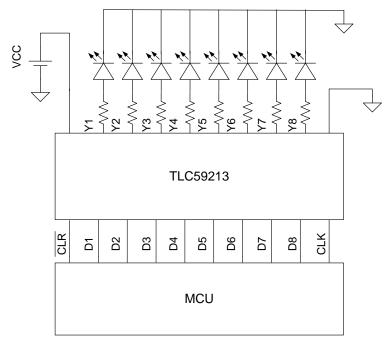
Figure 4. Typical Application Diagram
