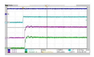
Figure 5. Output Voltage and Current Response
