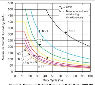
Figure 2. Maximum Output Current vs Duty Cycle (DIP (N) Package)
