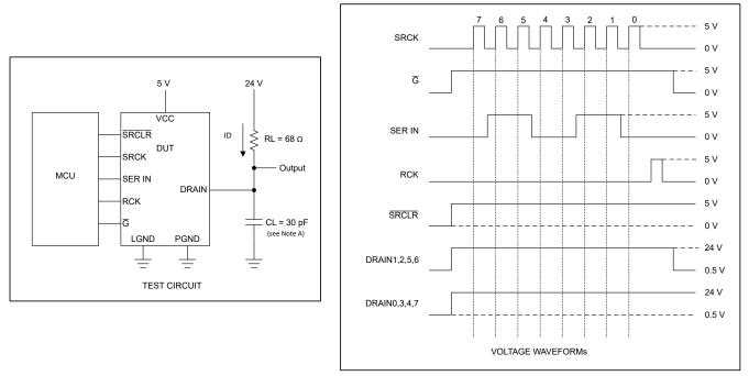
A. C<sub>L</sub> includes probe and jig capacitance.
