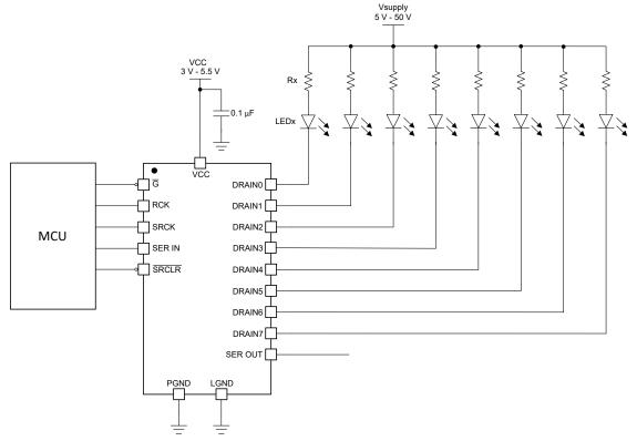
Figure 9-1. Typical Application With TLC6A598 to Drive LEDs
