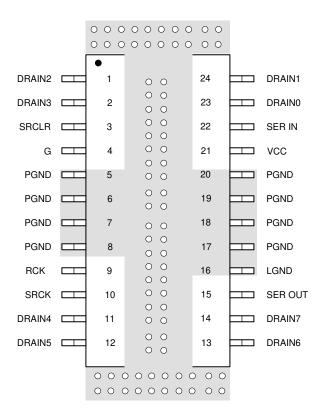
Figure 11-1. TLC6A598 Example Layout
