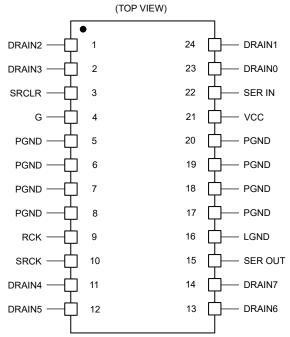
Figure 5-1. DW Package 24-Pin SOIC Top View
