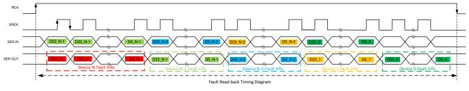
Figure 8-4. Register Read Timing Diagram
