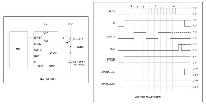
A. C<sub>L</sub> includes probe and jig capacitance.
