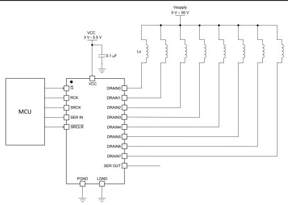
Figure 9-5. Typical Application With TLC6A598 to Drive Relays
