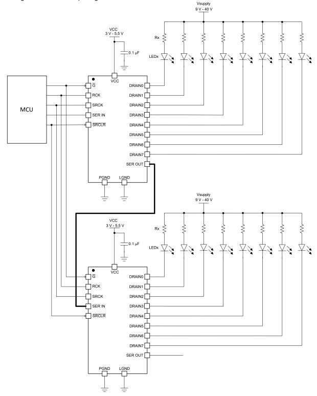
Figure 9-4. Typical Application With Cascade TLC6A598
