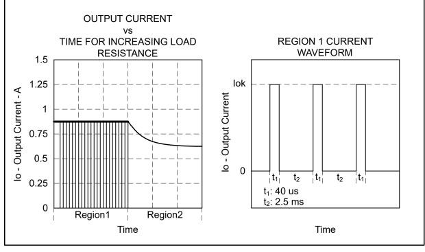
Figure 8-2. Chopping-Mode Characteristics
