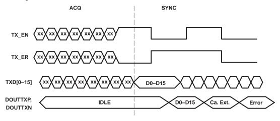
Figure 7. Transmit Side Timing Diagram
