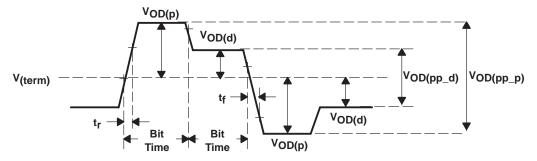
Figure 12. Differential and Common-Mode Output Voltage Definitions
