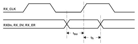
Figure 4. Receive Timing Waveform
