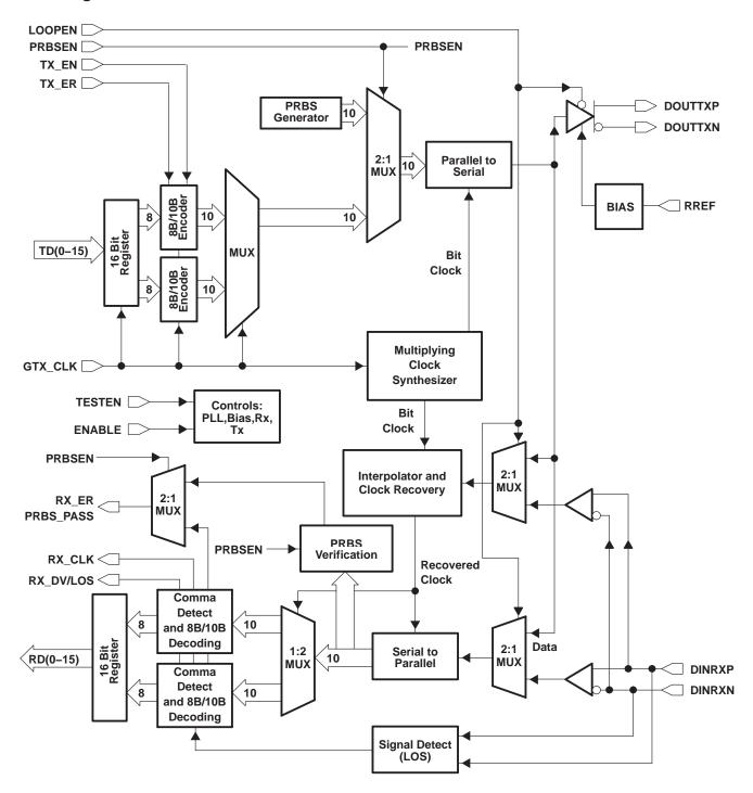
Figure 1. TLK1501 Block Diagram
