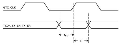
Figure 2. Transmit Timing Waveform
