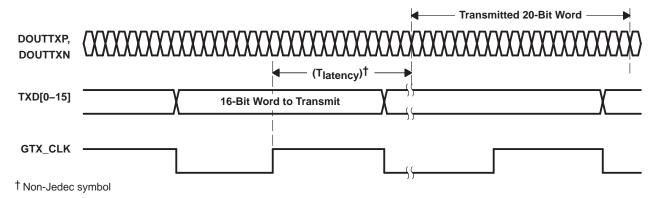
Figure 3. Transmitter Latency
