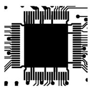
Figure 17. Example of a Thermal Land
