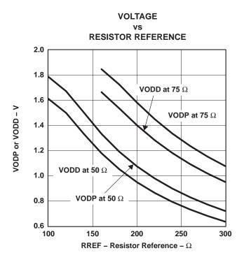
Figure 14. Differential Transmitter Voltage
