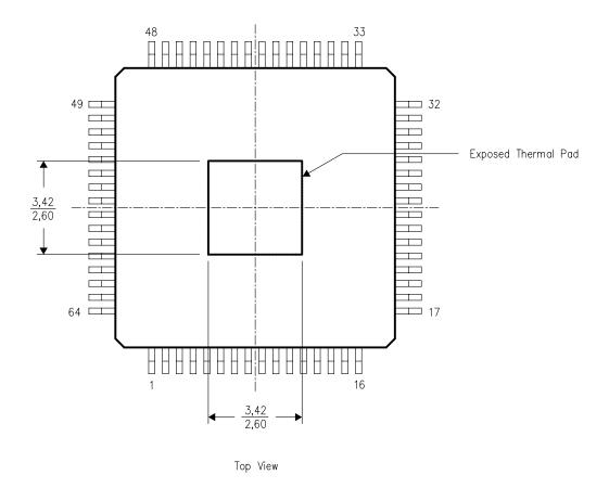
NOTE: All linear dimensions are in millimeters
