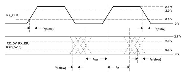
Figure 11. TTL Data Output Valid Levels for ac Measurements
