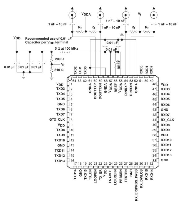
Figure 13. External Component Interconnection
