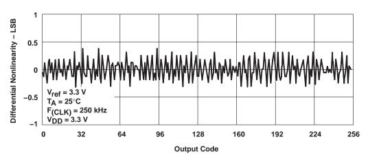
Figure 11. Differential Nonlinearity With Output Code
