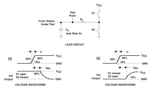
NOTE A:  $\ensuremath{\text{C}_{L}}$  includes probe and jig capacitance.
