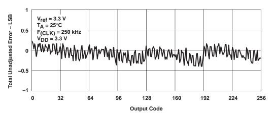
Figure 13. Total Unadjusted Error With Output Code
