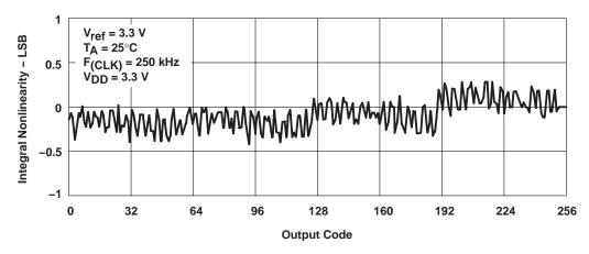
Figure 12. Integral Nonlinearity With Output Code
