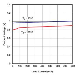
Figure 8-2. Dropout Voltage vs Load Current
