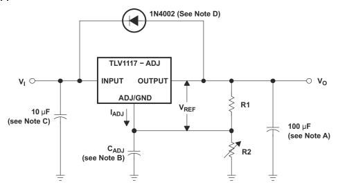
Figure 8-1. Basic Adjustable Regulator
