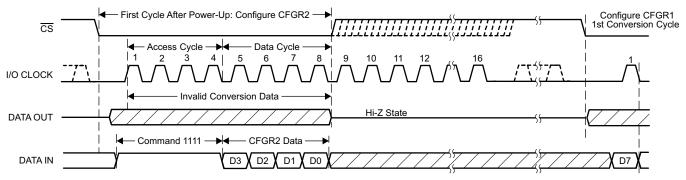
NOTE: To minimize errors caused by noise at  $\overline{\text{CS}}$ , the internal circuitry waits for a set-up time after the  $\overline{\text{CS}}$  falling edge before responding to control input signals. Therefore, no attempt should be made to clock in an address until the minimum  $\overline{\text{CS}}$  setup time has elapsed.
