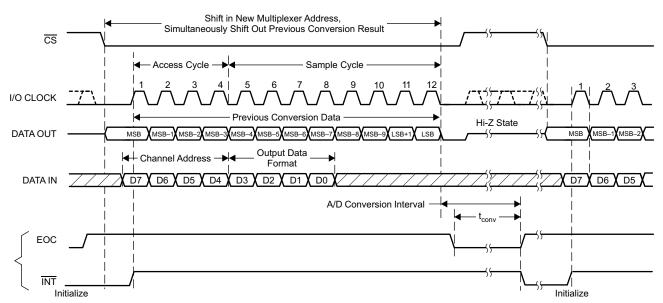
NOTE: To minimize errors caused by noise at  $\overline{\text{CS}}$ , the internal circuitry waits for a set-up time after the  $\overline{\text{CS}}$  falling edge before responding to control input signals. Therefore, no attempt should be made to clock in an address until the minimum  $\overline{\text{CS}}$  setup time has elapsed.
