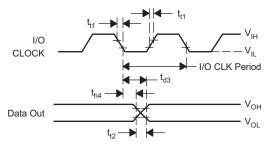
Figure 49. I/O CLOCK and DATA OUT Voltage **Waveforms**
