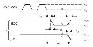
Figure 50. I/O CLOCK and EOC Voltage **Waveforms**
