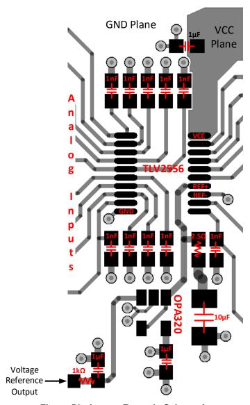
Figure 58. Layout Example Schematic
