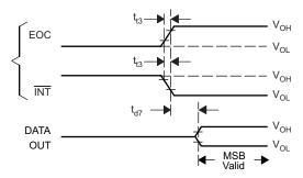
Figure 51. EOC and DATA OUT Voltage **Waveforms**
