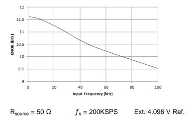
Figure 55. ENOB as a Function of Input Signal Frequency
