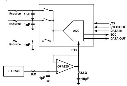
Figure 56. Typical Application Block Diagram
