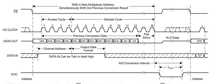
NOTE: To minimize errors caused by noise at  $\overline{\text{CS}}$ , the internal circuitry waits for a set-up time after the  $\overline{\text{CS}}$  falling edge before responding to control input signals. Therefore, no attempt should be made to clock in an address until the minimum  $\overline{\text{CS}}$  setup time has elapsed.
