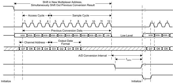
NOTE: To minimize errors caused by noise at  $\overline{CS}$ , the internal circuitry waits for a set-up time after the  $\overline{CS}$  falling edge before responding to control input signals. Therefore, no attempt should be made to clock in an address until the minimum  $\overline{CS}$  setup time has elapsed.
