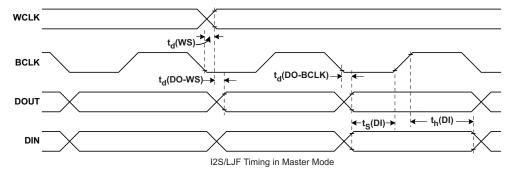
Figure 4. I<sup>2</sup>S/LJF/RJF Timing in Master Mode
