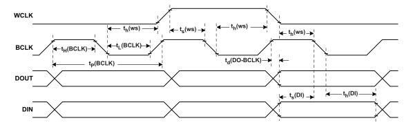
Figure 7. DSP Timing in Slave Mode
