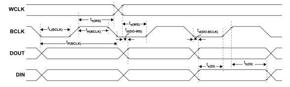
Figure 5. I<sup>2</sup>S/LJF/RJF Timing in Slave Mode
