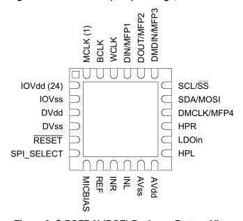
Figure 3. S-PQFP-N (RGE) Package, Bottom View
