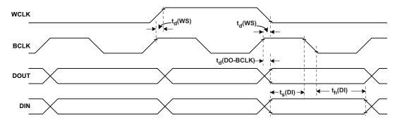
Figure 6. DSP Timing in Master Mode
