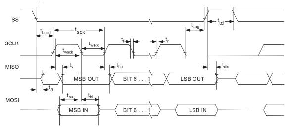
Figure 9. SPI Interface Timing Diagram
