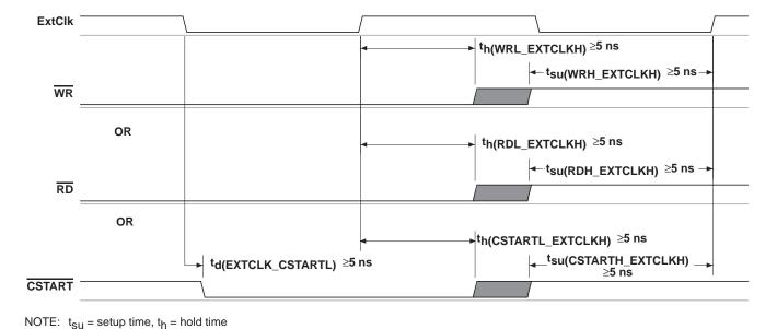
Figure 3. Trigger Timing – Software Start Mode Using External Clock
