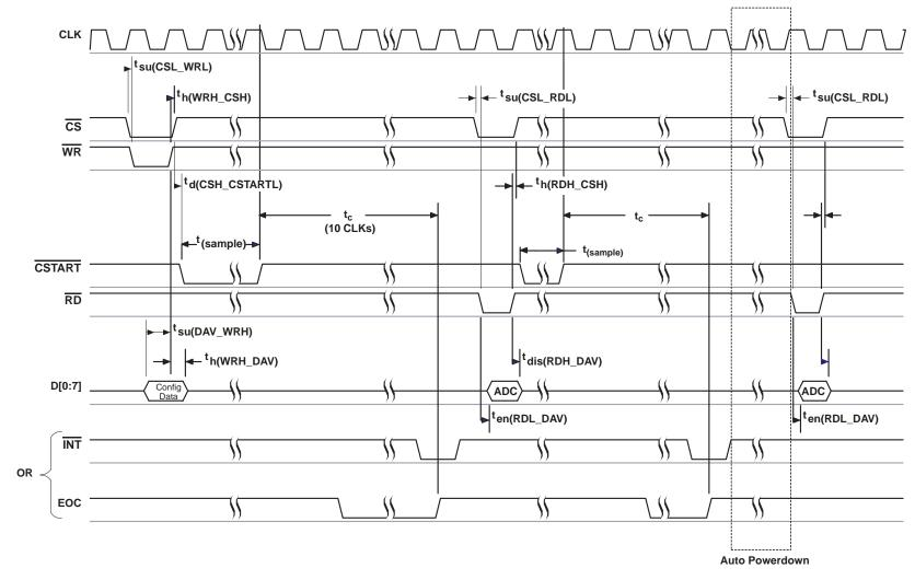
Figure 4. Input Conversion – Hardware CSTART, External Clock
