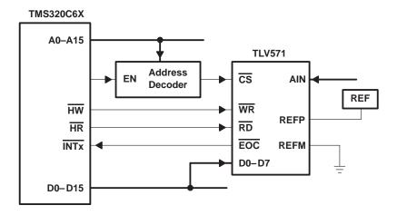
Figure 8. TMS320C6x DSP Interface
