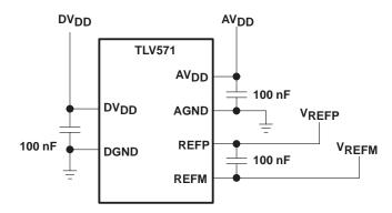
Figure 9. Placement for Decoupling Capacitors
