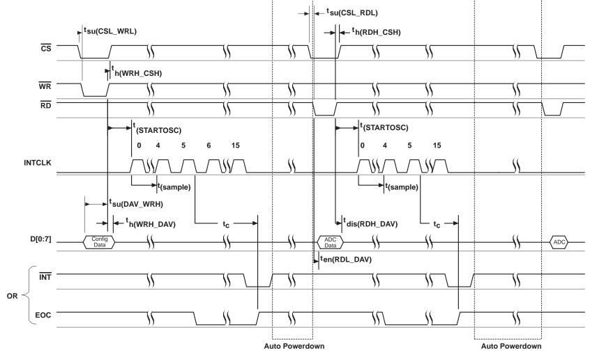
Figure 7. Input Conversion – Software Start, Internal Clock
