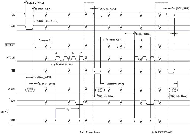
Figure 5. Input Conversion – Hardware CSTART, Internal Clock
