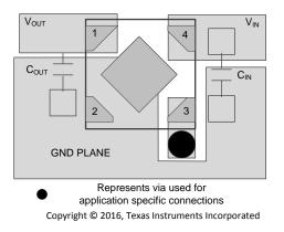
Figure 18. Recommended Layout Example
