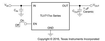
Figure 15. Typical Application Circuit
