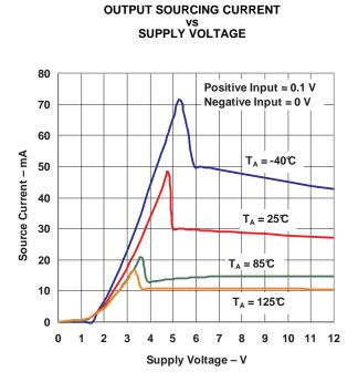
vs SUPPLY VOLTAGE 120 Positive Input = 0.1 V Negative Input = 0 V 100 80 T<sub>A</sub> = -40℃ 60
