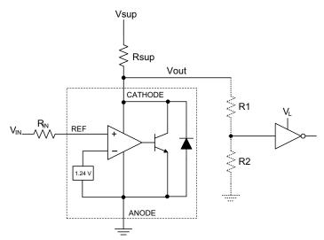
Figure 29. Comparator Application Schematic
