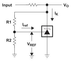
Figure 24. Test Circuit for  $V_{KA} > V_{REF}$ ,  $V_{O} = V_{KA} = V_{REF} \times (1 + R1 / R2) + I_{ref} \times R1$
