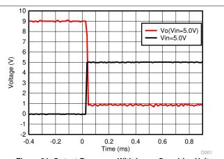
Figure 31. Output Response With Large Overdrive Voltage
