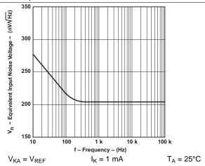
Figure 9. Equivalent Input Noise Voltage vs Frequency
