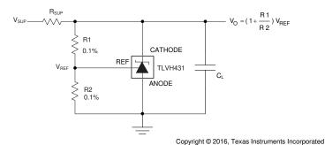
Figure 32. Shunt Regulator Schematic
