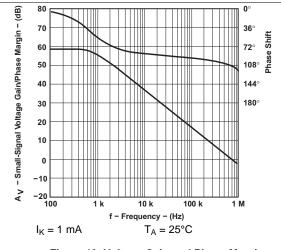
Figure 13. Voltage Gain and Phase Margin vs Frequency
