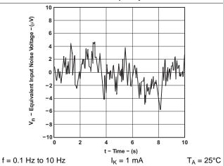
Figure 11. Equivalent Input Noise Voltage
