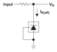
Figure 25. Test Circuit for I<sub>K(off)</sub>
