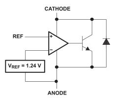
Figure 26. Equivalent Schematic
