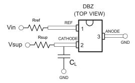
Figure 34. DBZ Layout Example
