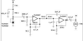
Figure 12. Test Circuit for 0.1-Hz to 10-Hz Equivalent Noise Voltage
