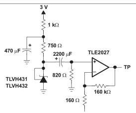
Figure 10. Test Circuit for Equivalent Noise Voltage
