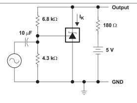
Figure 14. Test Circuit for Voltage Gain and Phase Margin
