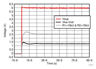
Figure 33. TLVH431B-EP Start-Up Response
