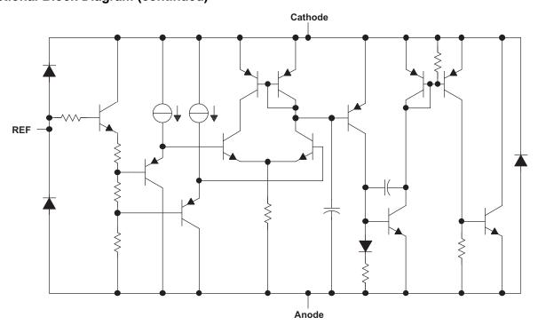
Figure 27. Detailed Schematic
