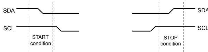
Figure 21-3. START and STOP Conditions
