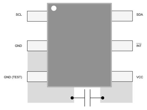
Figure 10-1. Layout Example With TMAG5273
