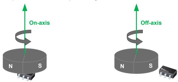
Figure 8-16. On-Axis vs. Off-Axis Angle Measurements
