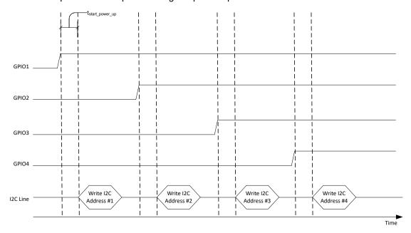
Figure 8-14. Power-Up Timing and I<sup>2</sup>C Address Allocation for the Four Sensors
