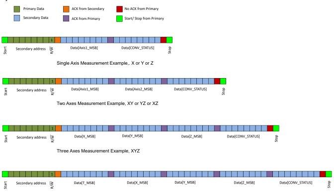
Figure 7-13. 1-Byte I<sup>2</sup>C Read Command for 8-Bit Data With CRC Disabled, CRC\_EN = 0b
