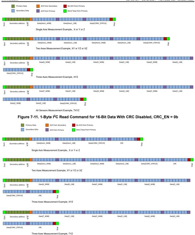
Figure 7-12. 1-Byte I<sup>2</sup>C Read Command for 16-Bit Data With CRC Enabled, CRC\_EN = 1b
