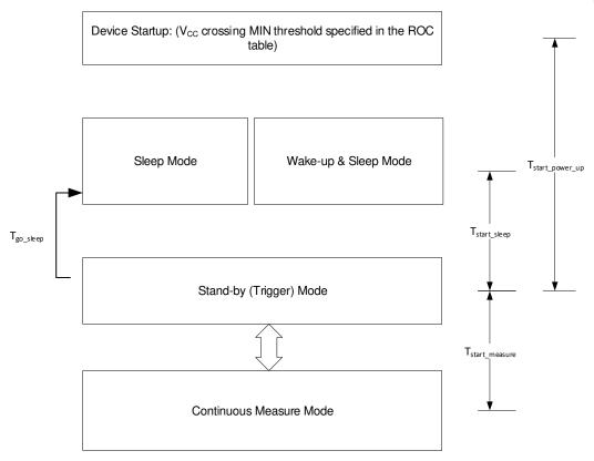
Figure 7-6. TMAG5273 Power-Up Sequence
