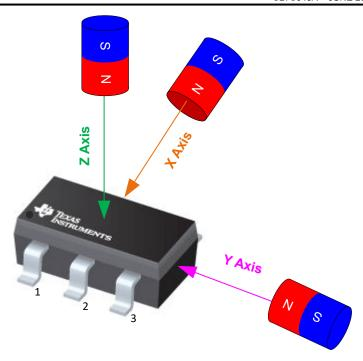
Figure 7-1. Direction of Sensitivity
