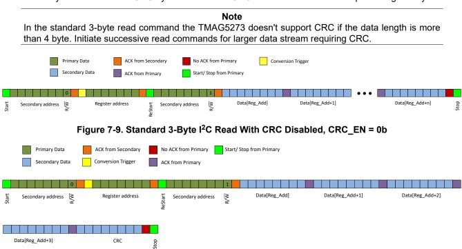
Figure 7-10. Standard 3-Byte I<sup>2</sup>C Read With CRC Enabled, CRC\_EN = 1b
