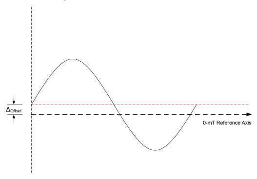
Figure 7-19. Magnetic Sensor Data Offset Correction
