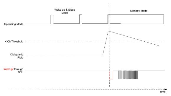
Figure 7-3. Interrupt Through SCL
