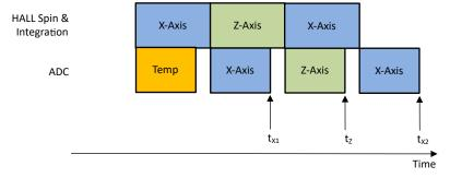
Figure 8-3. XZX Magnetic Field Conversion
