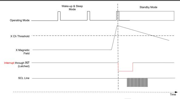
Figure 7-5. Latched Interrupt Through INT
