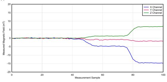
Figure 8-12. Tamper Detection During Continuous Conversion
