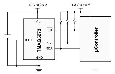
Figure 8-15. TMAG5273 Application Diagram for Angle Measurement
