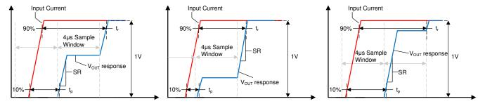
Figure 8-3. Small Current Input Step Transient Response
