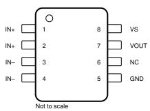
Figure 6-1. D Package 8-Pin SOIC Top View
