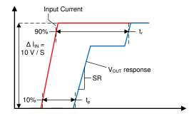
Figure 8-4. Current Overload Transient Response
