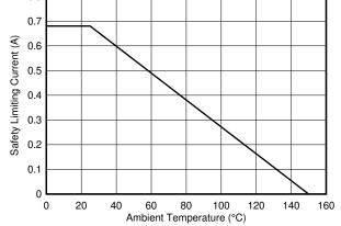
Figure 7-15. Thermal Derating Curve for Safety-Limiting Current, Side 2
