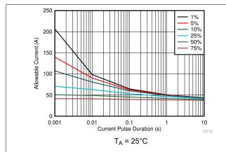
Figure 8-6. Maximum Repetitive Pulsed Current vs Pulse Duration
