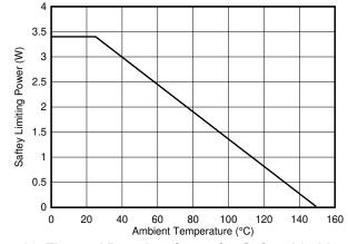
Figure 7-16. Thermal Derating Curve for Safety-Limiting Power
