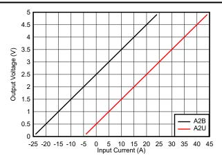
Figure 9-9. Output Voltage Relationship to Input Current for TMCS1108A2B and TMCS1108A2U
