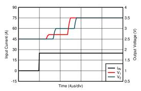
Figure 8-2. Transient Step Response
