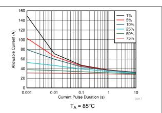
Figure 8-7. Maximum Repetitive Pulsed Current vs Pulse Duration
