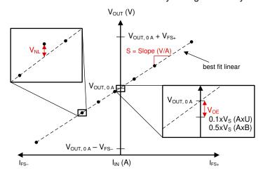
Figure 8-1. Sensitivity, Offset, and Nonlinearity Error
