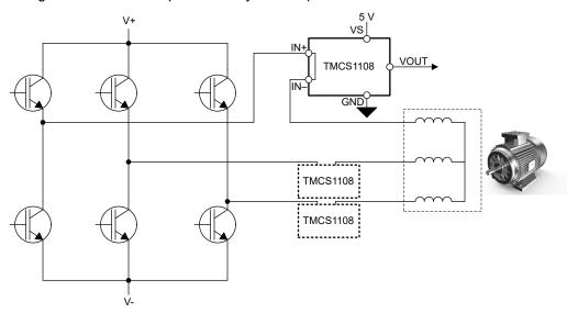
Figure 10-2. Inline Motor Phase Current Sensing
