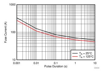
Figure 8-10. Single-Pulse Leadframe Capability
