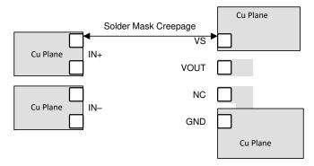
Figure 12-2. Layout for System Creepage Requirements
