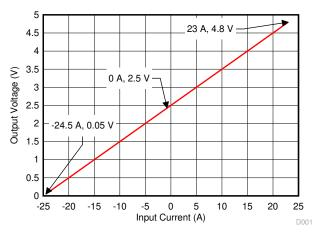
Figure 10-3. Application Example Design Transfer Curve
