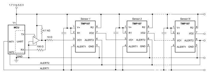
Figure 42. Connecting ALERT1 and ALERT2 Pins
