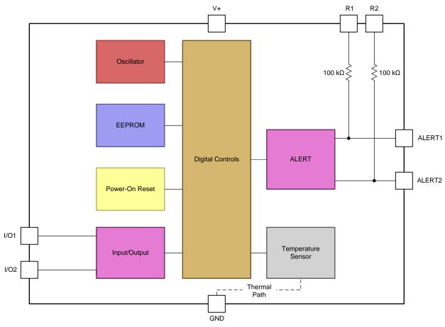
NOTE: The temperature sensor of the TMP107-Q1 is the silicon chip. Thermal paths run through the package leads. The lower thermal resistance of metal enables the leads to provide the primary thermal path.
