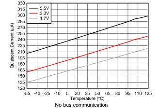
Figure 9. Continuous-Conversion Current vs Temperature
