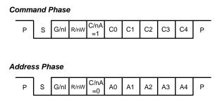
Figure 20. Command and Address Phase
