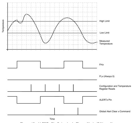
Figure 17. ALERTx Pin Behavior in Therm Mode (POLx = 0)
