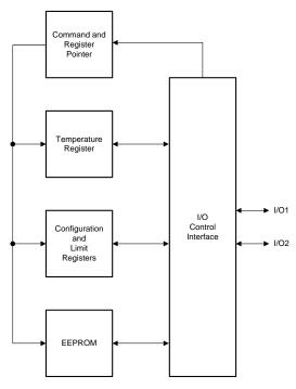
Figure 30. Register Structure
