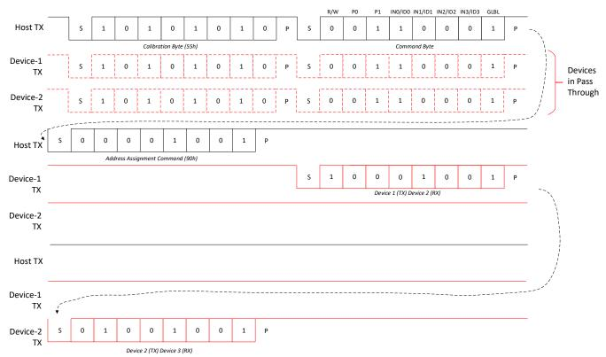
Figure 7-8. Global Initialization and Address Assignment Command Flow
