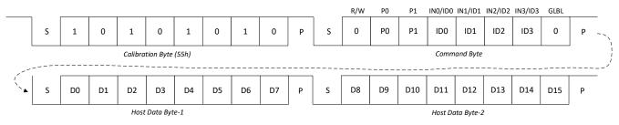
Figure 7-14. Individual Write Command Flow
