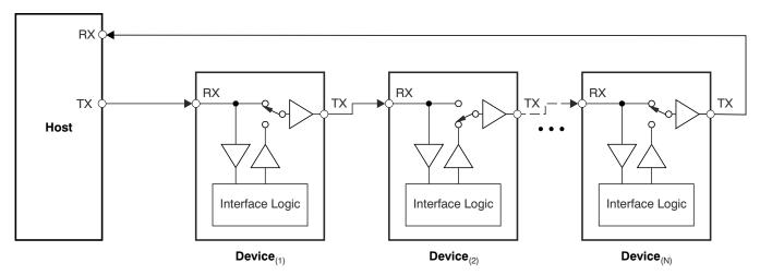
Figure 7-16. TMP144 Daisy-Chain: Bus Status During Individual Read Operation of Second Device
