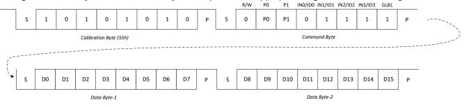
Figure 7-12. Global Write Command Flow
