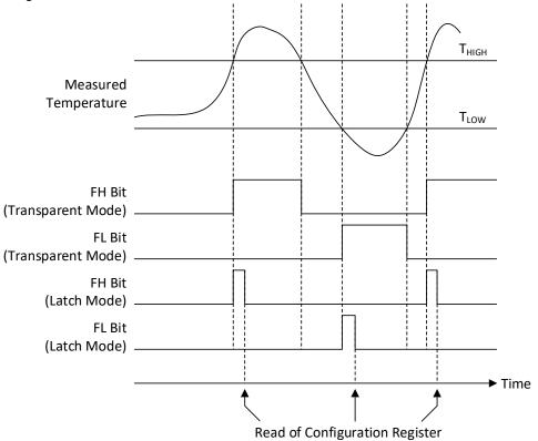
Figure 7-2. Temperature Flag Functional Diagram
