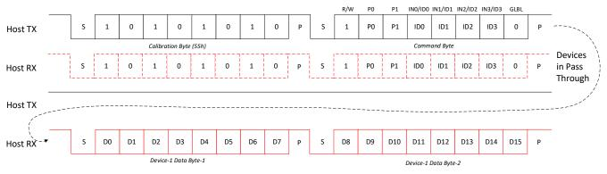
Figure 7-15. Individual Read Command Flow
