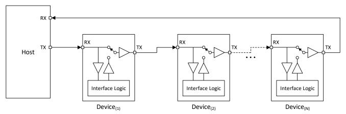
Figure 7-7. TMP144 Daisy-Chain: Bus Status at Start of Global Initialization
