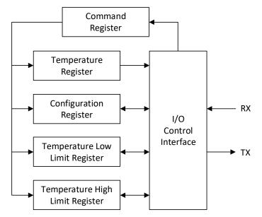
Figure 7-17. Internal Register Structure
