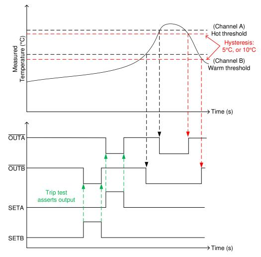
Figure 8. TMP392 Trip Test Operation
