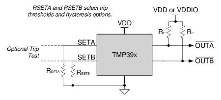
Figure 9. Simplified Schematic
