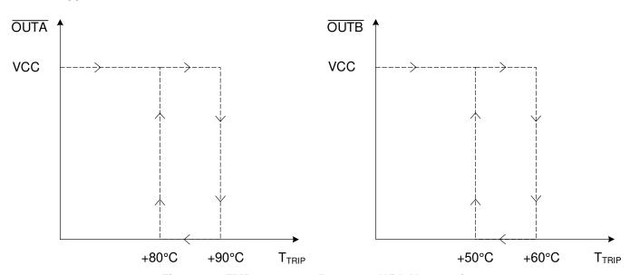
Figure 12. TMP392 Output Response With Hysteresis
