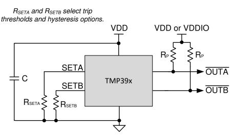
Figure 7. Simplified Schematic
