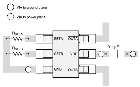
Figure 16. TMP392 Recommended Layout
