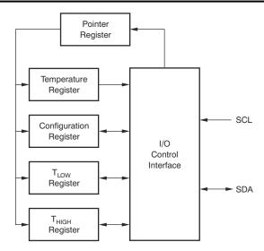
Figure 7-7. Internal Register Structure
