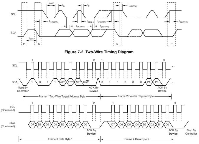
A. The value of A0, A1, and A2 are determined by the connections of the corresponding pins.
