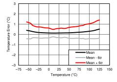
Temperature Accuracy (Error) vs. Ambient Temperature
