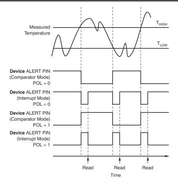
Figure 7-1. ALERT Pin Modes of Operation
