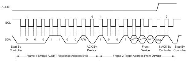
A. The value of A0, A1, and A2 are determined by the connections of the corresponding pins.
