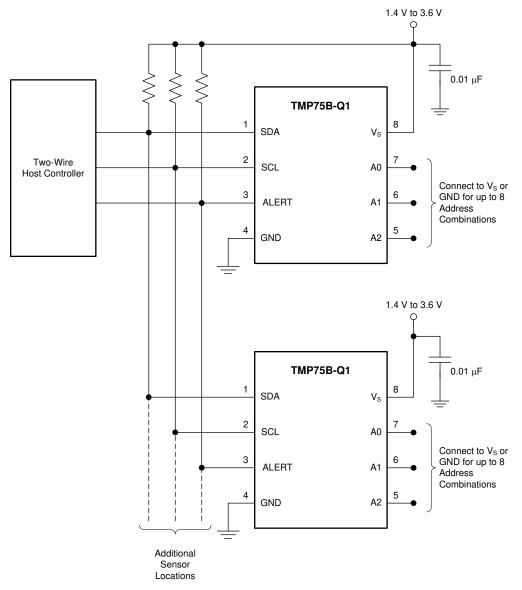
Figure 8-1. Temperature Monitoring of Multiple Locations on a PCB
