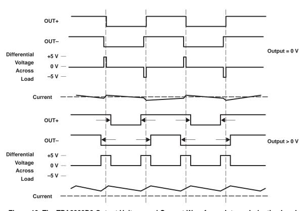
Figure 13. The TPA2000D2 Output Voltage and Current Waveforms Into an Inductive Load
