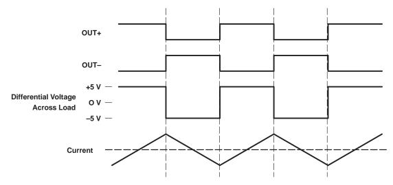
Figure 12. Traditional Class-D Modulation Scheme's Output Voltage and Current Waveforms Into an Inductive Load With No Input
