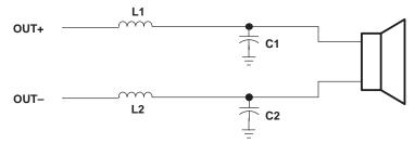
Figure 1. Class-D Output Filter
