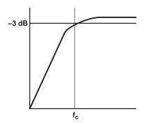
The value of  $C_l$  is important, as it directly affects the bass (low frequency) performance of the circuit. Consider the example where  $Z_l$  is 20 k $\Omega$  and the specification calls for a flat bass response down to 80 Hz. Equation 5 is reconfigured as Equation 6.
