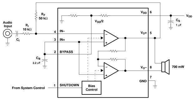
Figure 26. TPA721 Application Circuit
