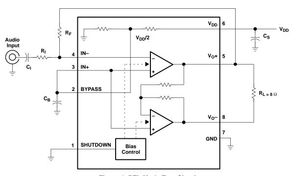
Figure 1. BTL Mode Test Circuit
