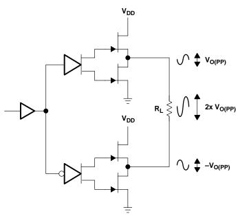
Figure 23. Bridge-Tied Load Configuration
