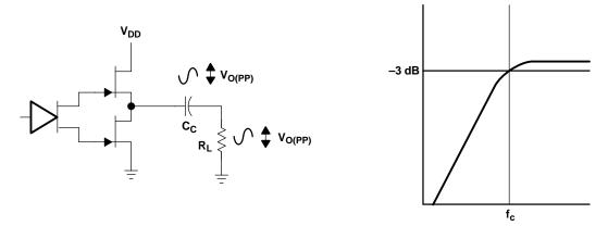
Figure 24. Single-Ended Configuration and Frequency Response
