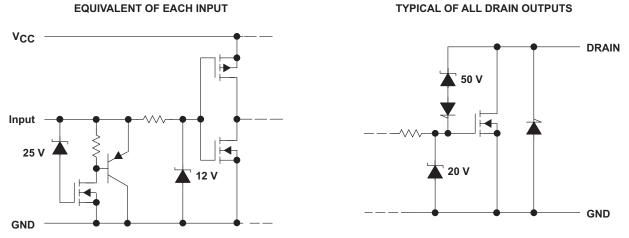
Figure 13. Schematic of Inputs
