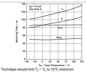
Figure 5. Switching Time vs Case Temperature
