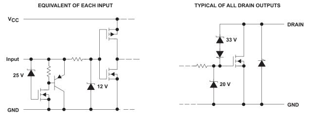
Figure 13. Schematic of Inputs and Outputs
