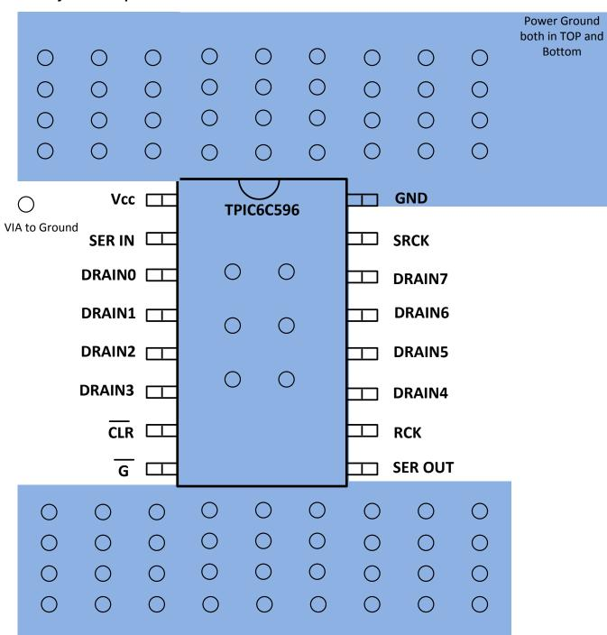
Figure 16. Recommended Layout Example
