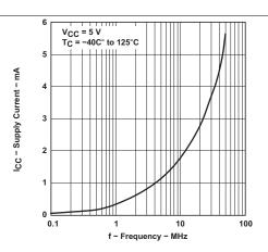
Figure 2. Supply Current vs Frequency
