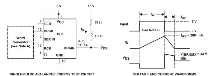
NOTES: A. The word generator has the following characteristics:  $t_r \le 10$  ns,  $t_f \le 10$  ns,  $t_O = 50$   $\Omega$ .
