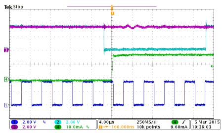
Figure 15. CH1 is SRCK, CH2 is RCK, CH3 is SER IN and CH4 is D1 Current
