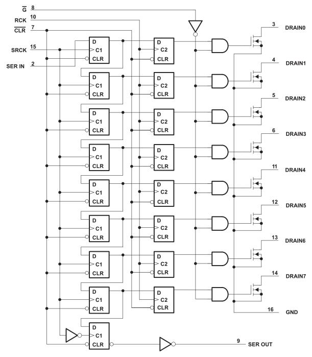
Figure 12. Logic Diagram (Positive Logic)
