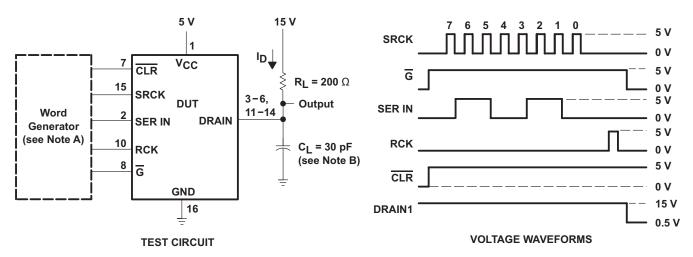
NOTES: A. The word generator has the following characteristics:  $t_{\Gamma} \le 10$  ns,  $t_{W} = 300$  ns, pulsed repetition rate (PRR) = 5 kHz,  $Z_{O} = 50 \ \Omega$ .
