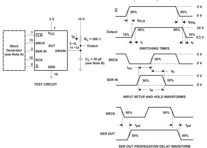
NOTES: A. The word generator has the following characteristics:  $t_{\Gamma} \le 10$  ns,  $t_{W} = 300$  ns, pulsed repetition rate (PRR) = 5 kHz,  $Z_{O} = 50 \ \Omega$ .
