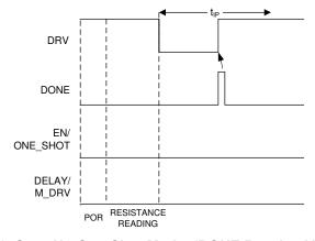
Figure 7-2. Start-Up One-Shot Mode, (DONE Received Within t<sub>IP</sub>)
