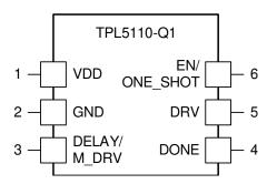
Figure 5-1. SOT-23 6-Lead DDC Top View
