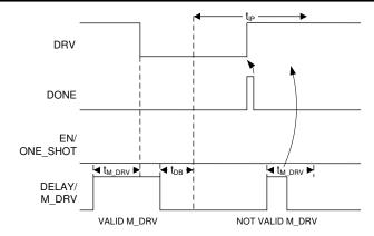
Figure 7-5. Manual MOSFET Power ON in One-Shot Mode
