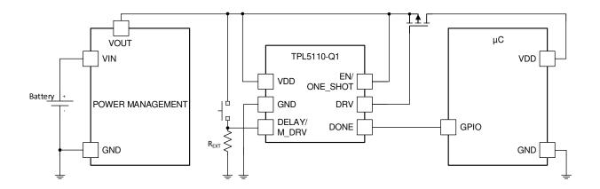
Figure 7-6. Manual MOSFET Power ON with SPST Switch
