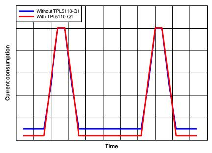
Figure 8-2. Effect of TPL5110-Q1 on Current Consumption
