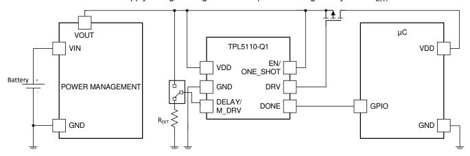
Figure 7-7. Manual MOSFET Power ON with SPDT Switch
