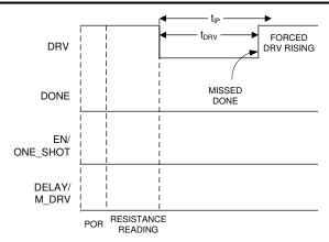
Figure 7-3. Start-Up One-Shot Mode, (No DONE Received Within t<sub>IP</sub>)
