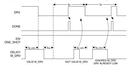
Figure 7-4. Manual MOSFET Power ON in Timer Mode
