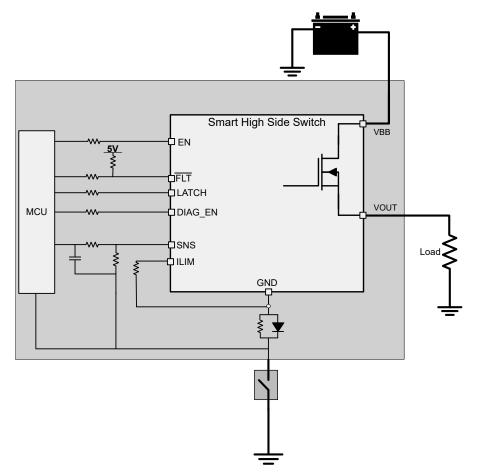
Figure 8-20. Loss of Module GND
