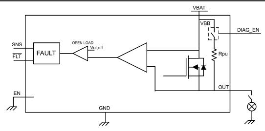
Figure 8-16. Open-Load Detection Circuit
