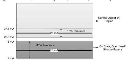
Figure 8-15. On-State Open-Load Detection and Normal-Operation Diagram
