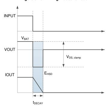
Figure 8-11. Inductive-Load Switching-Off Diagram
