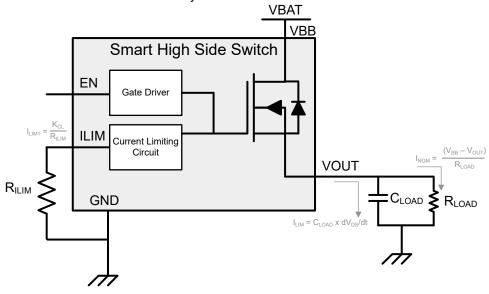
Figure 8-8. Capacitive Charging Circuit
