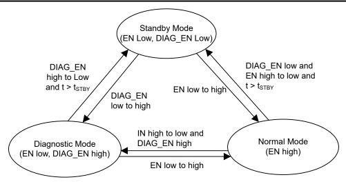
Figure 8-25. Work Mode State Machine
