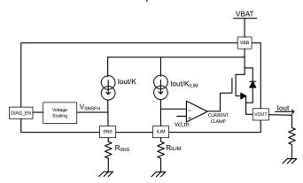
Figure 8-3. Current-Sense and Current-Limit Block Diagram
