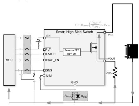
Figure 8-23. Reverse Protection with GND Network
