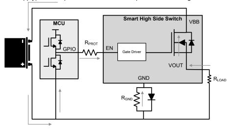
Figure 8-17. Reverse Battery Circuit
