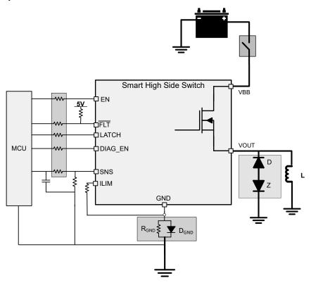
Figure 8-21. Loss of Battery
