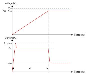
Figure 8-9. Capacitive Charging Timing
