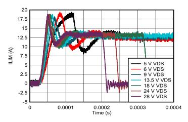
Figure 8-6. Current Limit Regulation With Varying VDS, RILIM = 7.15 k $\Omega$
