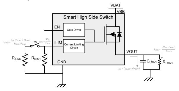
Figure 9-2. Dynamic Changing Current Limit Setup
