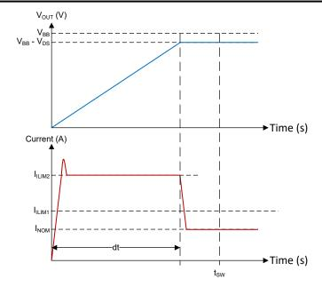
Figure 9-3. Capacitive Charging Changing Current Limit
