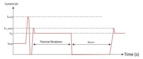
Figure 8-13. On-State Short-Circuit Behavior
