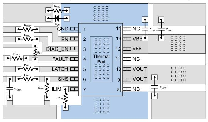
Figure 9-6. Layout With a GND Network
