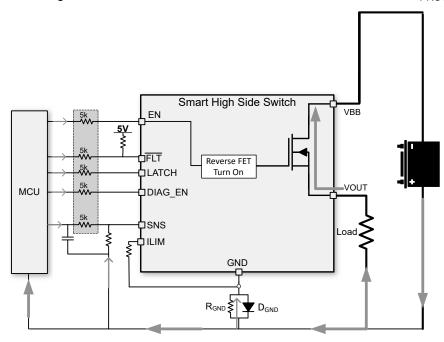
Figure 8-24. MCU I/O Protections
