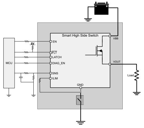
Figure 8-19. Loss of Device GND
