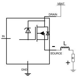
Figure 8-10. Driving Inductive Load
