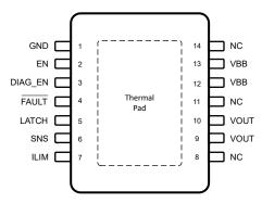
Figure 5-1. PWP Package, 14-Pin HTSSOP (Top View)
