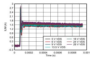
Figure 8-5. Current Limit Regulation With Varying VDS, RILIM = 71.5 k $\Omega$
