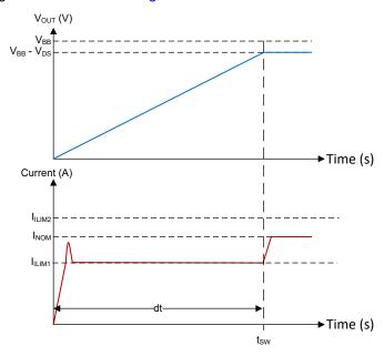
Figure 9-4. Large Capacitive Charging Changing Current Limit
