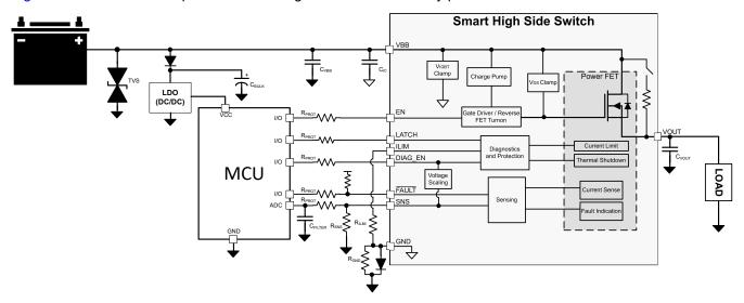
Figure 9-1. Typical Application Circuitry
