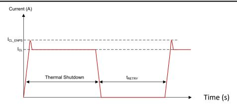
Figure 8-12. Enable into Short-Circuit Behavior (LATCH=0)
