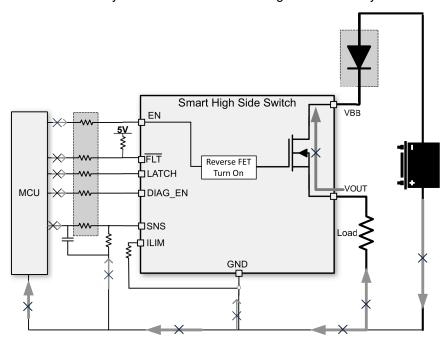
Figure 8-22. Reverse Protection with Blocking Diode
