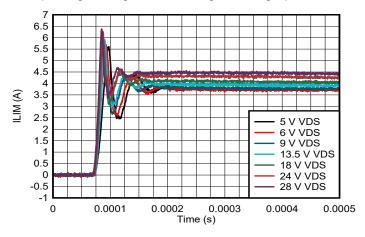
Figure 8-4. Current Limit Regulation With Varying VDS, RILIM = 25 k $\Omega$
