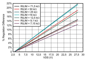
Figure 8-7. Current Limit Regulation Percentage Change With Varying V<sub>DS</sub>
