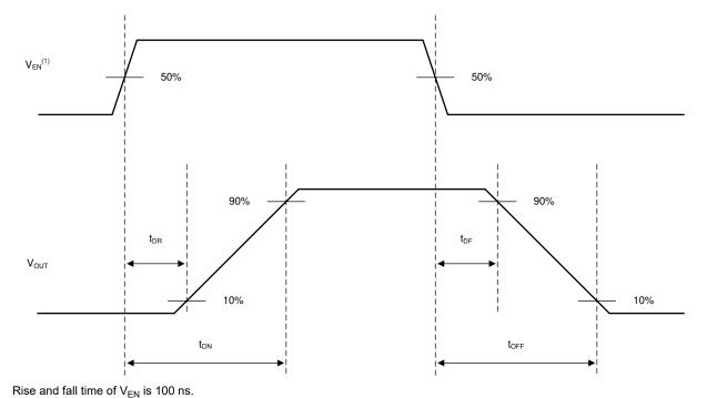
Figure 7-2. Switching Characteristics Definitions
