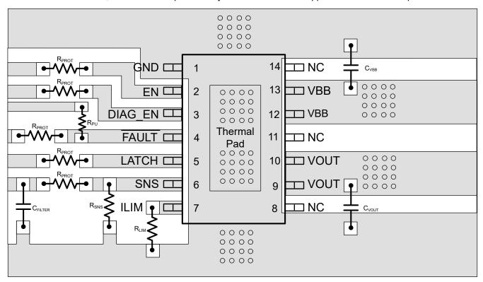
Figure 9-5. Layout Without a GND Network
