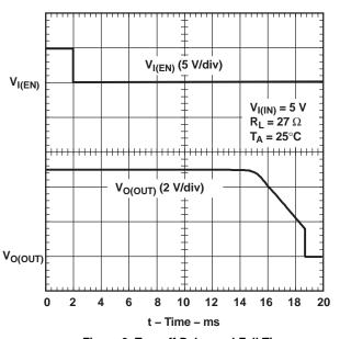
Figure 3. Turnoff Delay and Fall Time
