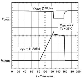
Figure 11. TPS2034, Ramped Load on Enabled Device
