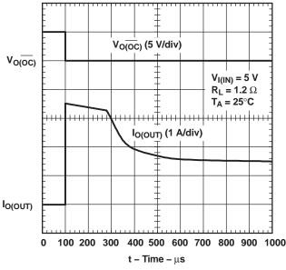
Figure 18. 1.2-Ω Load Connected to an Enabled TPS2032 Device
