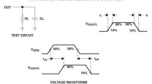
Figure 1. Test Circuit and Voltage Waveforms
