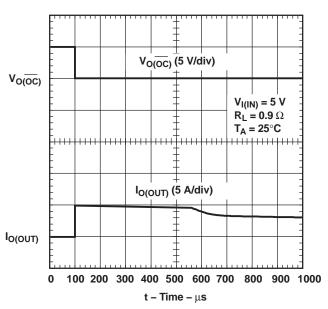
Figure 21. 0.9-Ω Load Connected to an Enabled TPS2034 Device
