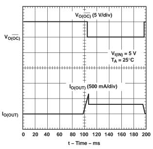
Figure 7. TPS2030, Ramped Load on Enabled Device
