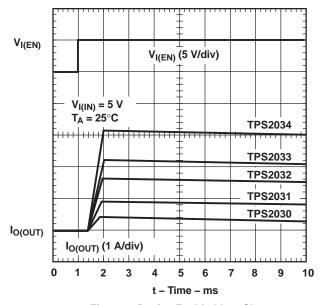
Figure 6. Device Enabled Into Short
