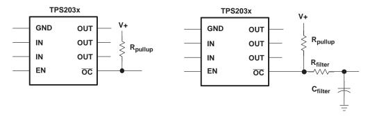
Figure 39. Typical Circuit for OC Pin and RC Filter for Damping Inrush OC Responses
