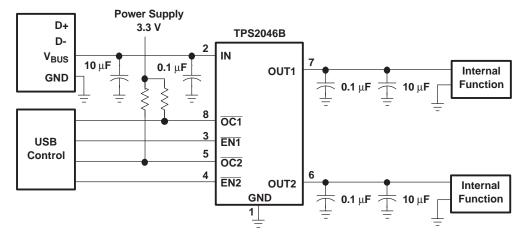
Figure 25. High-Power Bus-Powered Function (Example, TPS2046B)
