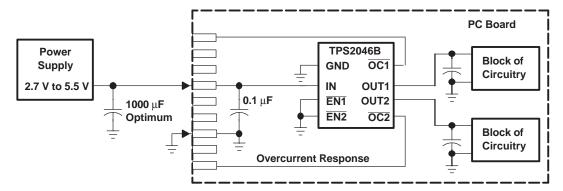
Figure 28. Typical Hot-Plug Implementation (Example, TPS2046B)
