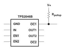
Figure 24. Typical Circuit for the OC Pin (Example, TPS2046B)
