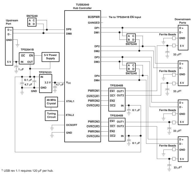
Figure 26. Hybrid Self/Bus-Powered Hub Implementation, TPS2046B
