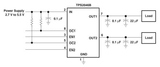
Figure 23. Typical Application (Example, TPS2046B)
