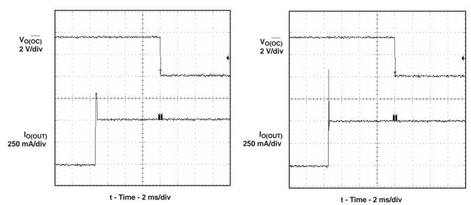
Figure 8. 4-Ω Load Connected to Enabled Device
