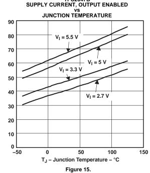
I (IN) – Supply Current, Output Enabled –  $\mu\text{A}$
