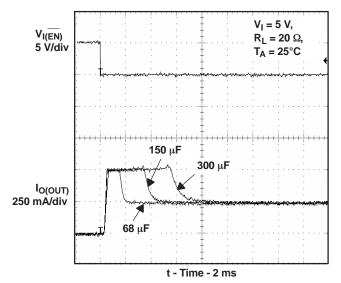
Figure 7. Inrush Current With Different Load Capacitance
