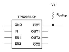
Figure 22. Typical Circuit for the OC Pin
