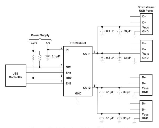
Figure 23. Typical Four-Port USB Host / Self-Powered Hub
