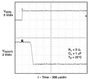
Figure 2. Turnon Delay and Rise Time With 1-µF Ĺoad
