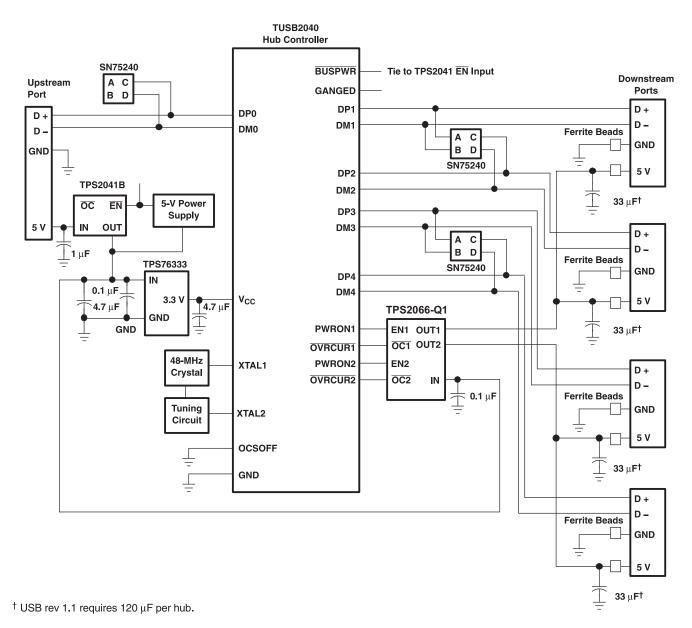
Figure 25. Hybrid Self / Bus-Powered Hub Implementation
