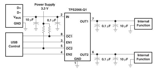
Figure 24. High-Power Bus-Powered Function
