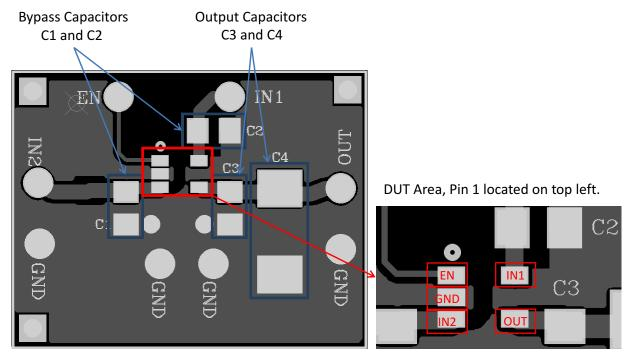
Figure 20. Input and Output Capacitors and DUT Area
