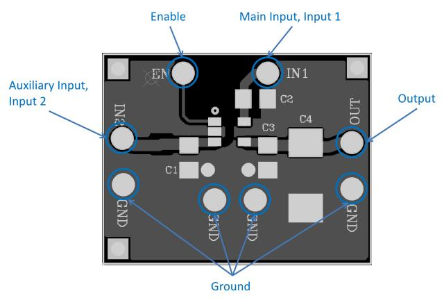
Figure 21. Enable, Input, Output, and Ground Pins
