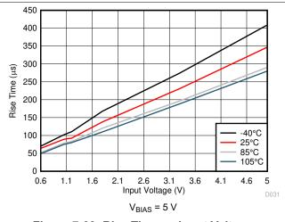
Figure 7-38. Rise Time vs Input Voltage
