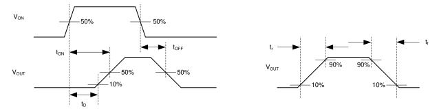
Figure 8-2.  $t_{ON}$  and  $t_{OFF}$  Waveforms
