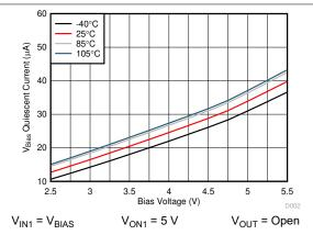
Figure 7-2. V<sub>BIAS</sub> Quiescent Current vs Bias Voltage Single Channel (TPS22976, TPS22976N)
