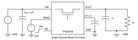
Figure 8-1. Test Circuit
