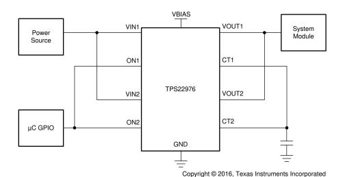
Figure 10-1. Parallel Configuration
