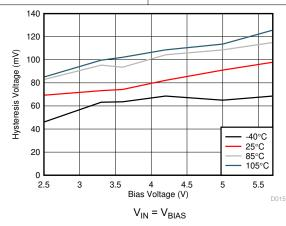
Figure 7-15. Voltage Input Hysteresis vs Bias Voltage
