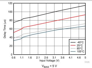
Figure 7-34. Delay Time vs Input Voltage
