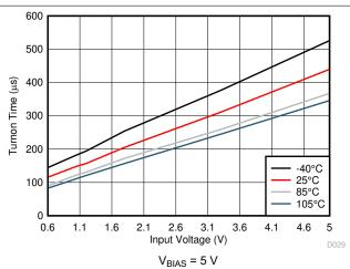
Figure 7-36. Turnon Time vs Input Voltage
