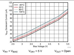
Figure 7-4. V<sub>BIAS</sub> Quiescent Current vs Bias Voltage Single Channel (TPS22976A)
