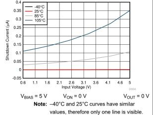
Figure 7-6. Off-State V<sub>IN</sub> Current vs Input Voltage **Single Channel**
