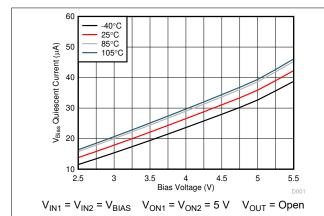
Figure 7-1. V<sub>BIAS</sub> Quiescent Current vs Bias Voltage Both Channels (TPS22976, TPS22976N)
