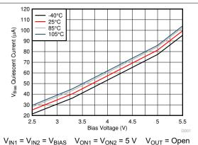
Figure 7-3. V<sub>BIAS</sub> Quiescent Current vs Bias Voltage Both Channels (TPS22976A)
