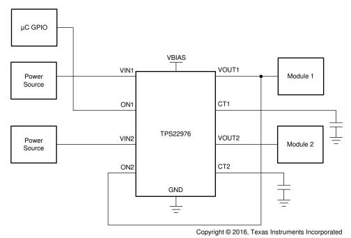
Figure 10-3. Power Sequencing without a GPIO Input
