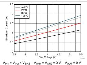
Figure 7-5. V<sub>BIAS</sub> Shutdown Current vs Bias **Voltage Both Channels**
