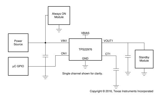
Figure 10-2. Standby Power Reduction
