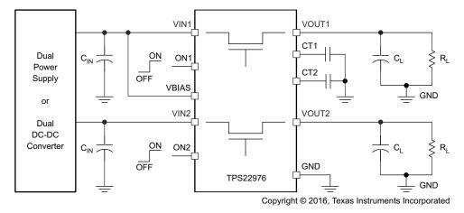
Figure 10-5. Typical Application Circuit
