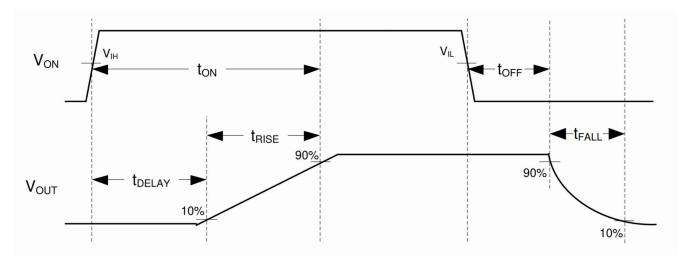
Figure 6-1. TPS22998 Timing Diagram
