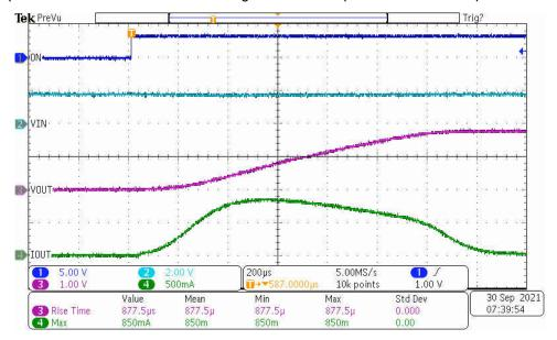
Figure 8-2. TPS22998 Turn-On into 470  $\mu$ F (CT =  $V_{BIAS}$ )
