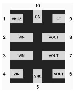
Figure 5-1. TPS22998 RYZ Package, 10-Pin WQFN (Top View)
