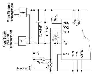
Figure 34. Low-Voltage Option 1 ORing
