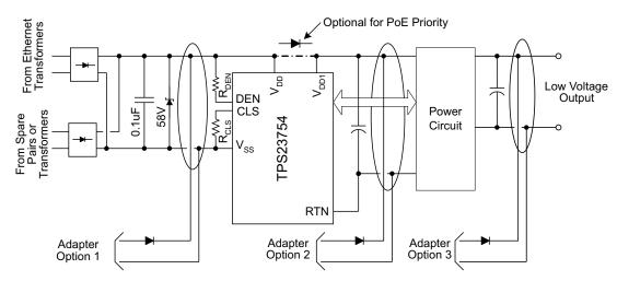
Figure 26. ORing Configurations
