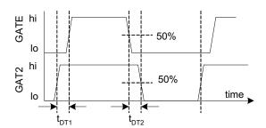
Figure 1. GATE and GAT2 Timing and Phasing
