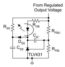
Figure 35. Error Amplifier Soft Start
