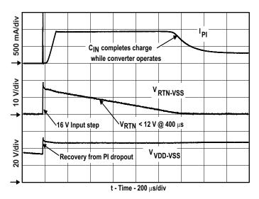
Figure 25. Response to PSE Step Voltage
