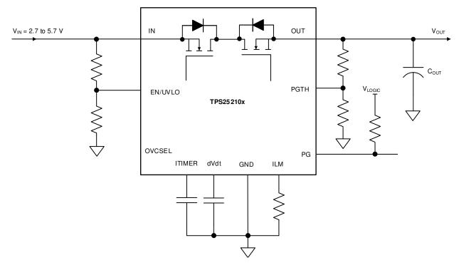
Figure 9-1. Single Device, Self-Controlled
