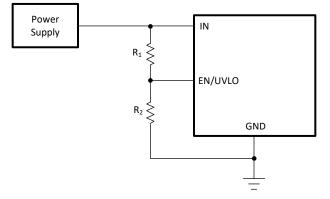
Figure 8-1. Adjustable Undervoltage Protection
