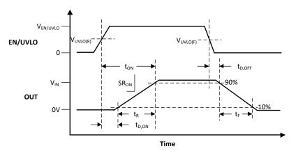
Figure 7-1. TPS2521xx Switching Times
