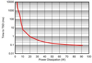
Figure 9-4. Thermal Shut-Down Plot During Inrush
