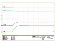
$V_{IN}$  = 5 V,  $C_{OUT}$  = 220 µF,  $R_{ILM}$  = 750  $\Omega$ ,  $I_{OUT}$  stepped up from 0 A to 4 A
