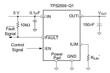
Figure 16. Typical TPS2559-Q1 Power Switch
