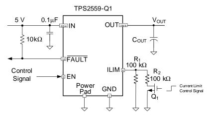
Figure 20. Two-Level Current-Limit Circuit
