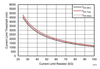
Figure 17. Current-Limit vs R<sub>(ILIM)</sub>
