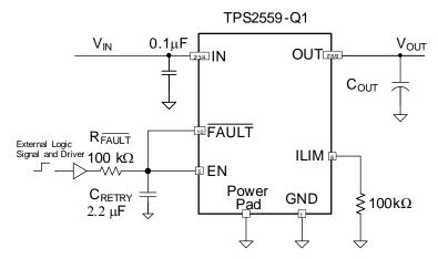
Figure 19. Auto-Retry Circuit with External EN Signal
