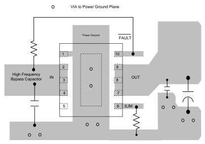
Figure 31. TPS2559-Q1 Board Layout
