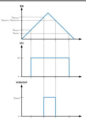
Figure 10-2. Precision Enable Behavior
