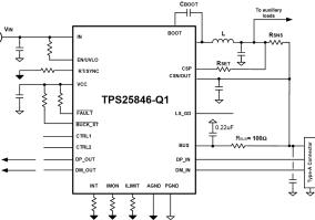
Figure 10-16. Current Limit with External MOSFET
