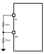
Figure 10-3. System UVLO by Enable Divider
