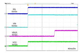
Figure 10-4. Typical Start-up Behavior,  $V_{IN}$  = 13.5 V,  $R_{IMON}$  = 12.6 k $\Omega$
