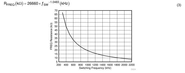
Figure 10-5. RT Set Resistor vs Switching Frequency
