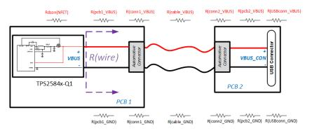
$$\label{eq:rescaled} \begin{split} R(wire) &= R(pcb1_VBUS) + R(conn1_VBUS) + R(cable_VBUS) + R(conn2_VBUS) + R(pcb2_VBUS) + R(USBconn_VBUS) + R(USBconn_GND) + R(pcb2_GND) + R(conn2_GND) + R(cable_GND) + R(conn1_GND) + R(pcb1_GND) + R(pcb$$
