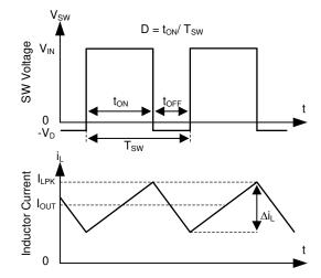
Figure 10-1. SW Node and Inductor Current Waveforms in Continuous Conduction Mode (CCM)
