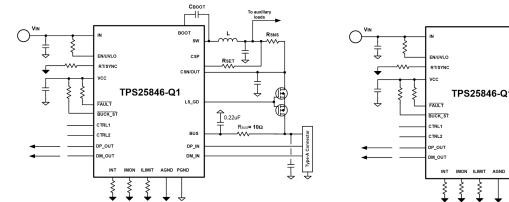
Figure 10-14. Current Limit with External MOSFET
