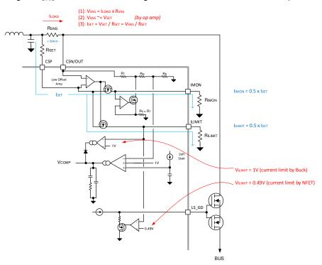
Figure 10-13. Current Limit and Cable Compensation Circuit
