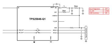
Figure 10-20. Client-Mode Equivalent Circuit
