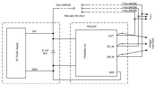
Figure 9-3. Short-to-Battery System Test Set-up
