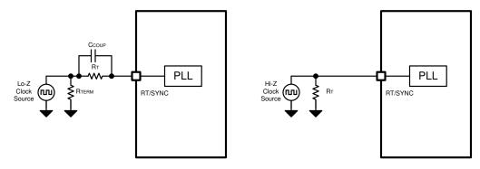
Figure 10-6. Synchronize to External Clock
