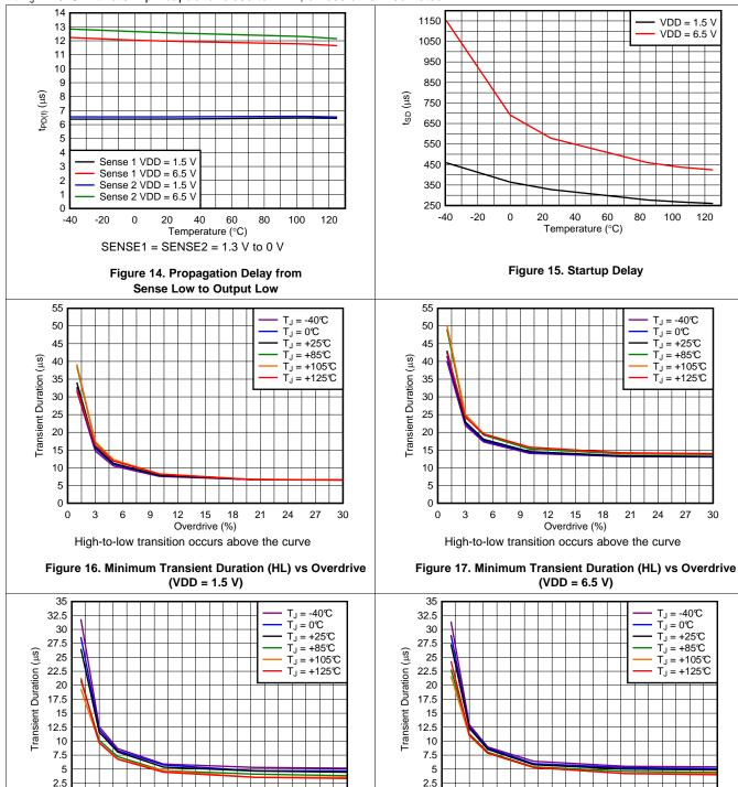
Figure 18. Minimum Transient Duration (LH) vs Overdrive (VDD = 1.5 V)
