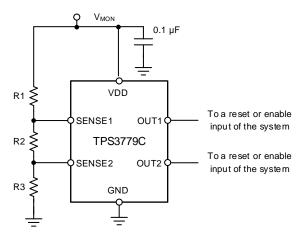
Figure 24. Early Warning Detection Schematic
