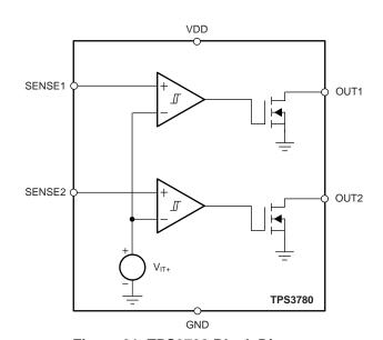
Figure 21. TPS3780 Block Diagram
