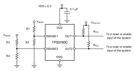
Figure 22. Monitoring Two Separate Rails Schematic
