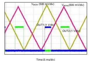
Figure 23. Monitoring Two Separate Rails Curve
