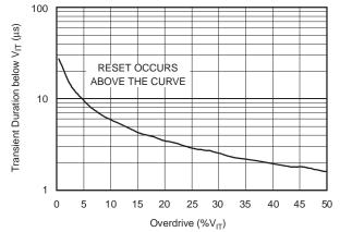
Figure 14. Maximum Transient Duration at Sense vs Sense Threshold Overdrive Voltage
