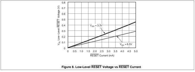
At T<sub>J</sub> = +25°C, V<sub>DD</sub> = 3.3 V, R<sub>LRESET</sub> = 100k $\Omega$ , and C<sub>LRESET</sub> = 50pF, unless otherwise noted.
