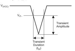
Figure 11. Voltage Transient Measurement
