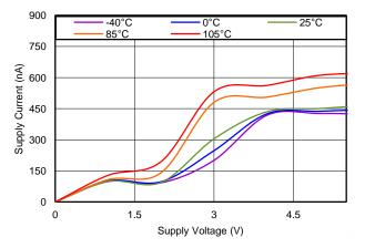
Figure 13. Supply Current During Startup
