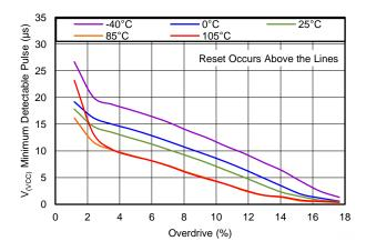
Figure 12. Minimum Detectable Pulse on VCC vs Overdrive
