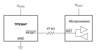
Figure 16. Connection to Bidirectional Reset Pin
