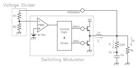
Figure 37. Linearizing the Modulator
