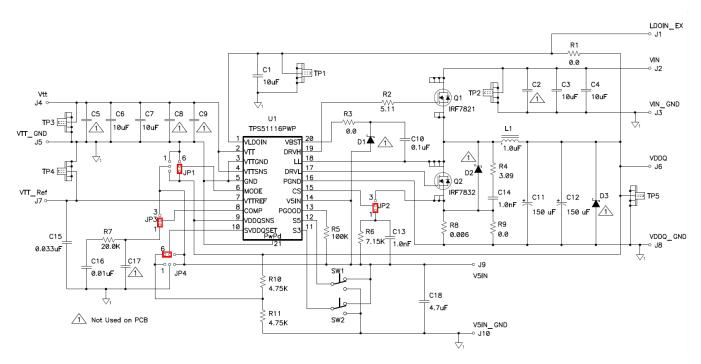
Figure 38. DDR3 Current Mode Application Schematic
