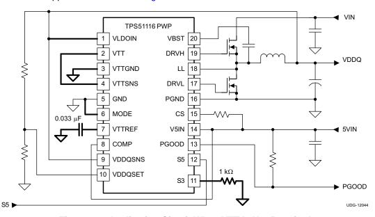
Figure 34. Application Circuit When VTT Is Not Required
