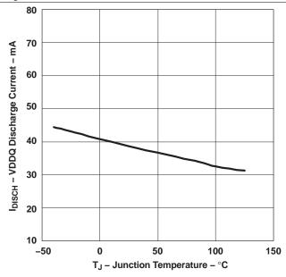
Figure 5. CS Current vs Junction Temperature
