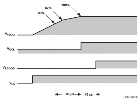
Figure 35. VDDQ Soft-Start and Powergood Timing
