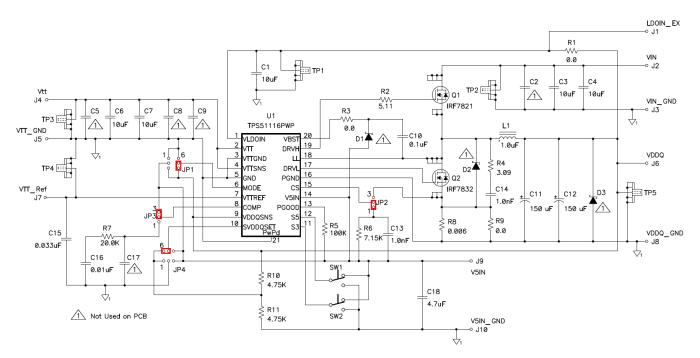
Figure 43. DDR3 DCAP Mode Application Schematic
