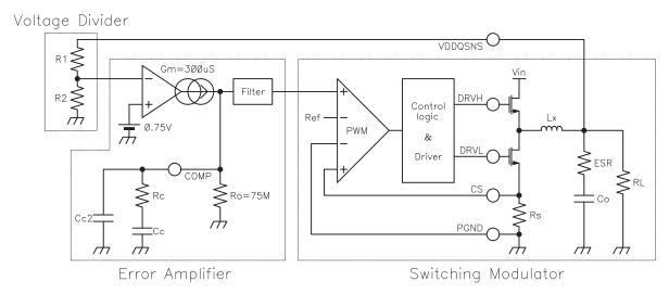
Figure 36. Linearizing the Modulator
