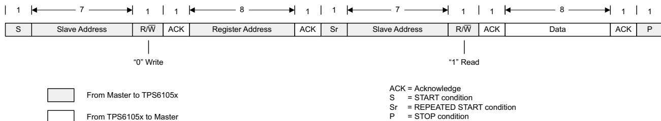
Figure 34. Read Data Transfer Format In F/S-Mode
