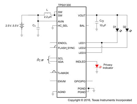
Figure 87. TPS61300 Typical Application Circuit
