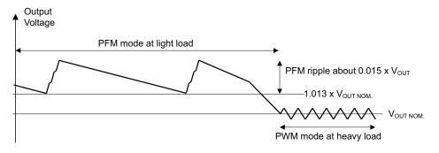
Figure 45. Operation in PFM Mode and Transfer to PWM Mode
