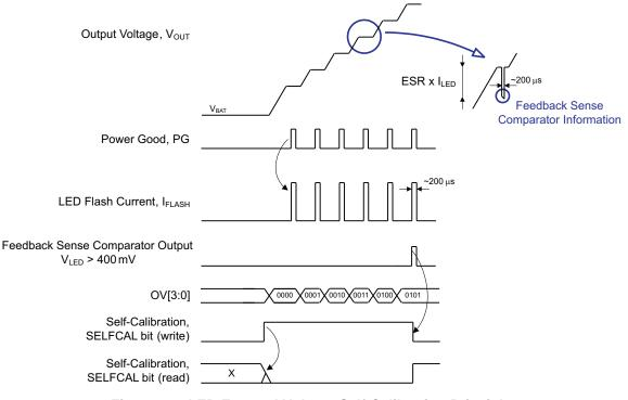
Figure 42. LED Forward Voltage Self-Calibration Principle
