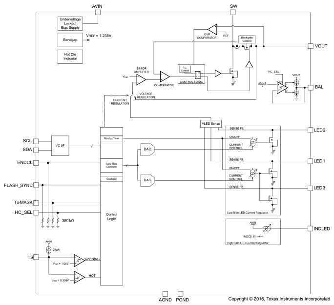
Figure 33. TPS61306 Block Diagram
