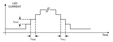
Figure 44. LED Current Slew-Rate Control
