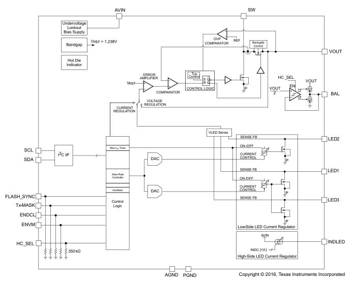
Figure 30. TPS61300 Block Diagram
