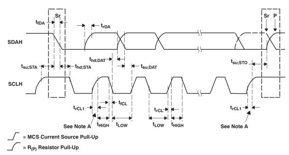
Note A: First rising edge of the SCLH signal after Sr and after each acknowledge bit.
