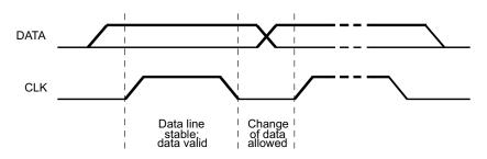
Figure 55. Bit Transfer On the Serial Interface
