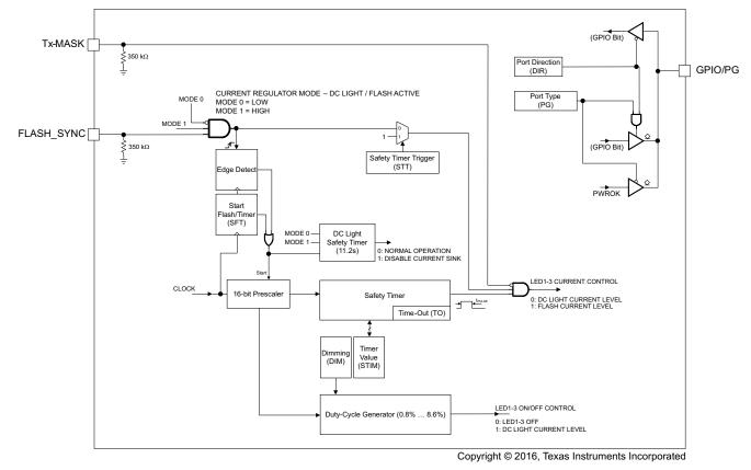
Figure 34. Timer Block Diagram Block Diagram
