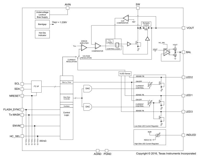
Figure 31. TPS61301 Block Diagram
