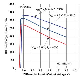
Figure 36. Typical DC Precharge and Short-Circuit Current
