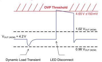
Figure 35. Overvoltage Protection Operation (4.65-V Typical)
