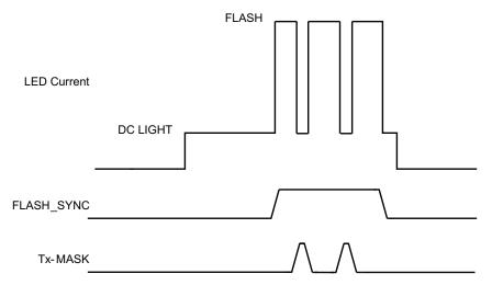
Figure 38. Synchronized Flashlight With Blanking Periods
