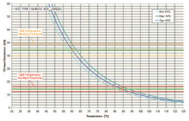
Figure 74. Temperature Monitoring Characteristic
