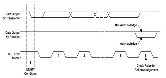
Figure 56. Acknowledge On the I<sup>2</sup>C Bus
