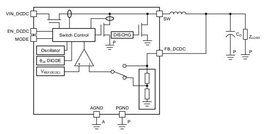
Figure 16. DC-DC Converter Block Diagram
