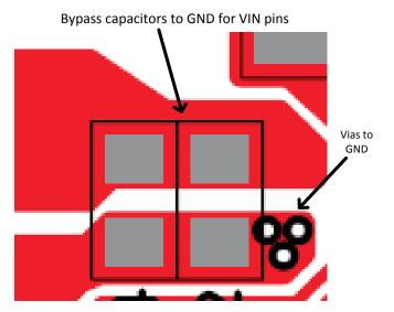
Figure 29. Bypass Capacitor and Via Placement Recommendation
