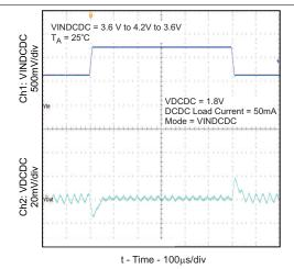
Figure 23. Line Transient Response (DC-DC PWM Mode)
