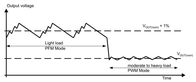
Figure 17. PFM Voltage Positioning
