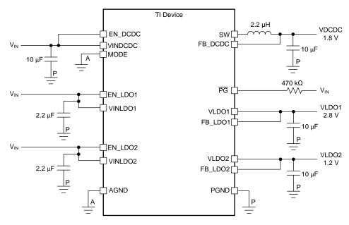
Figure 21. Typical Fixed Voltage Application Schematic
