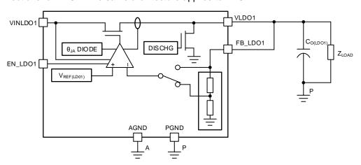
Figure 19. LDO Block Diagram
