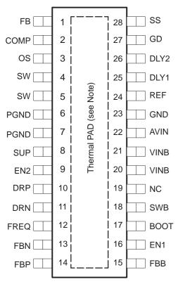
NOTE: The thermally enhanced PowerPAD<sup>™</sup> is connected to PGND.
