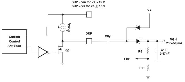
Figure 16. Extract of the Positive Charge-Pump Driver
