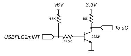
Figure 5. Circuit for Level-Shifting and Inverting nINT Signal
