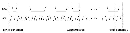
Figure 7. I<sup>2</sup>C Start / Stop / Acknowledge Protocol
