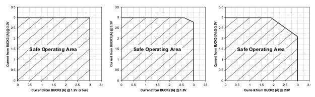
For any voltage / current comination inside the shaded area, the dissipated power inside the chip is below the allowable maximum. The examples assume  $T_{ambient}$  < 60°C,  $\eta$  = 90% and  $\theta_{JA}$  < 44°C/W.
