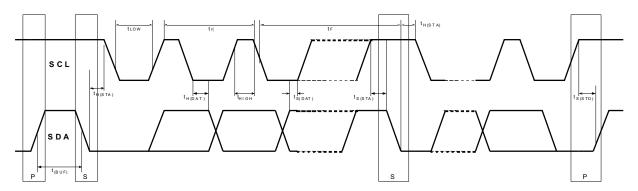
Figure 8. I<sup>2</sup>C Data Transmission Timing
