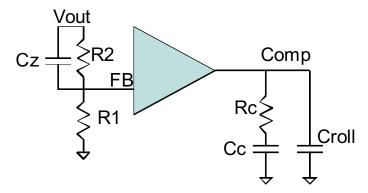
Figure 11. External Compensation Circuit
