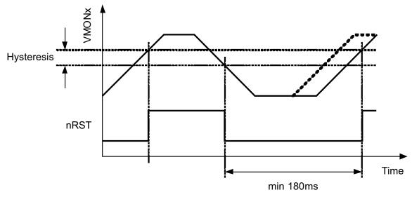
Figure 1. Supply Voltage Supervisor Reset Generation
