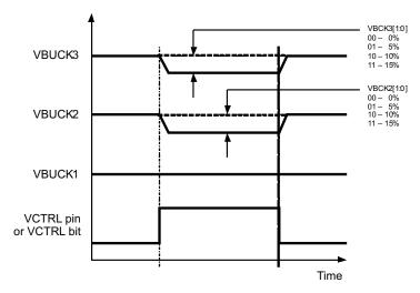
Figure 4. BUCK2 and BUCK3 Output Voltages
