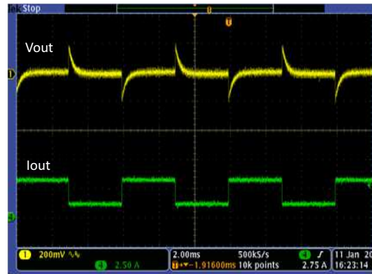
Figure 19. Buck Output Load Transient I_{OUT} = 1\text{ A} - 3\text{ A}
