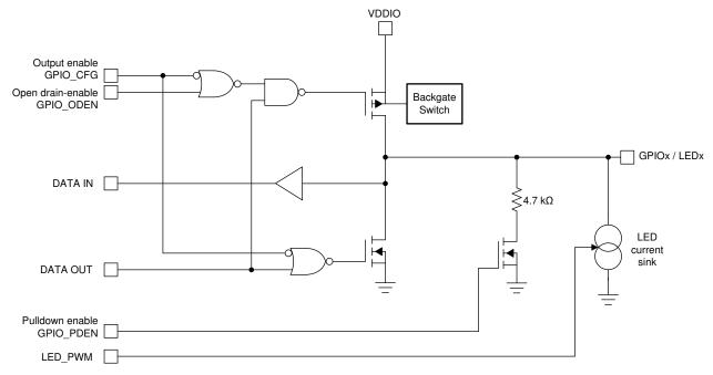
Figure 8-2. GPIO Block for GPIO3, GPIO4, and GPIO5
