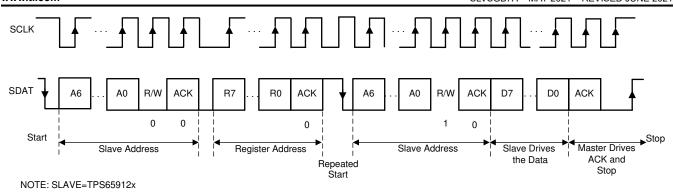
Figure 8-24. I<sup>2</sup>C Interface READ from TPS659128x; F/S Mode
