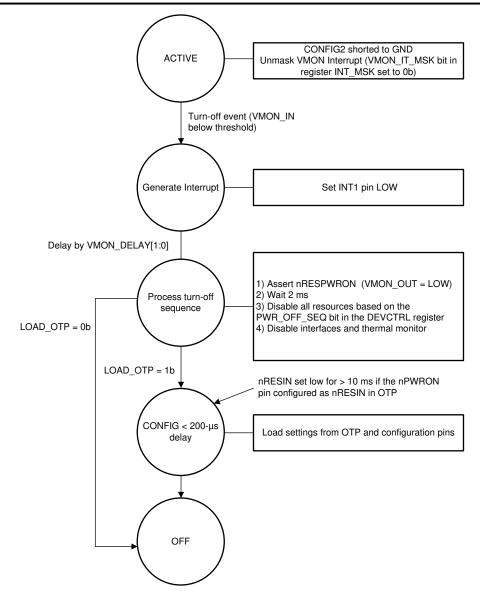
Figure 8-8. SHUTDOWN Flow for CONFIG2 Pin Shorted to GND
