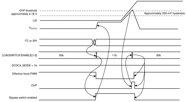
A. OVP enable = LOADSWITCH:ENABLE[1:0] = 10b or 11b LOADSWITCH:ENABLE[1] = 0b  $\rightarrow$  OVP enable = OVP = 0 If OVP hysteresis  $< V_{DCDC4} < OVP$  when LOADSWITCH:ENABLE[1] goes high, OVP indicates  $V_{DCDC4} < OVP$
