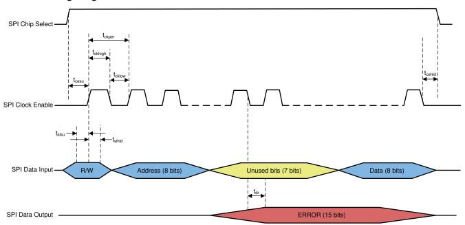
Figure 7-3. SPI Timing
