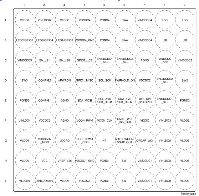
Figure 5-1. 81-Pin YFF DSBGA (Bottom View)
