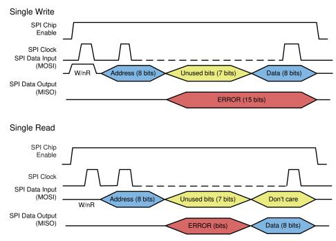
Figure 8-17. SPI READ and WRITE Protocol
