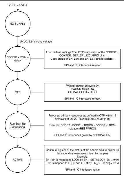
Figure 8-4. STARTUP Flow for CONFIG2 Pin Shorted to LDOAO
