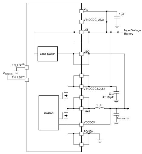
A. The EN LS1 pin must be high and the EN LS0 pin must be low to auto-enable the load switch based on the comparator in DCDC4.
