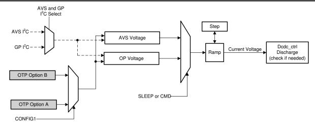
Figure 8-11. DC-DC Voltage Scaling Architecture
