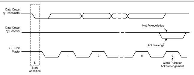
Figure 8-21. Acknowledge on the I<sup>2</sup>C Bus
