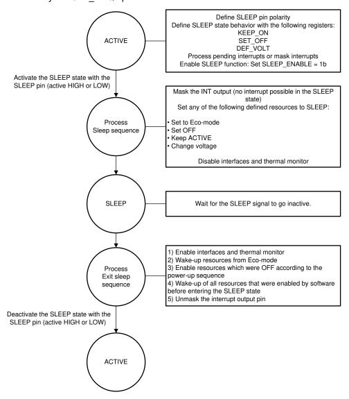
Figure 8-6. SLEEP Flow for CONFIG2 Pin Shorted LDOAO
