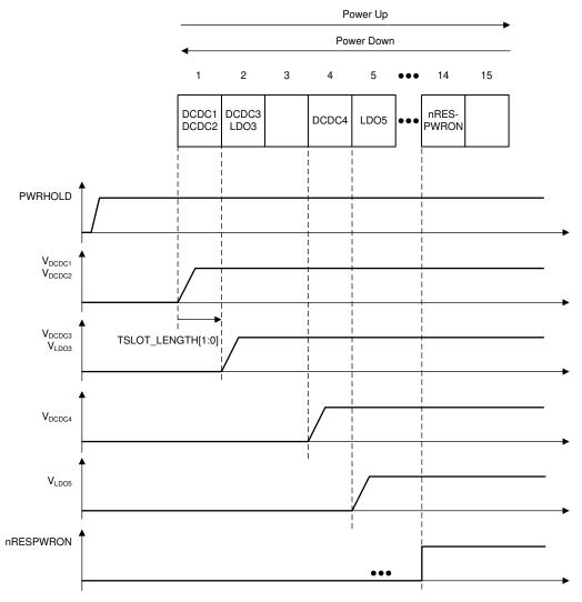
Figure 8-9. Internal Power-Up Example
