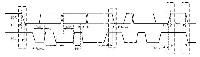
Figure 7-1. Serial Interface Timing Diagram for FS-Mode
