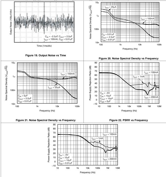
Figure 23. PSRR vs Frequency
