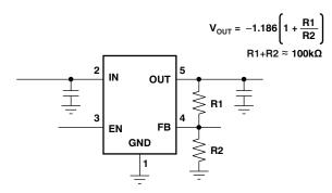
Figure 24. TPS72301-Q1 Adjustable LDO Regulator Programming
