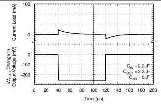
Figure 14. Load Transient Response
