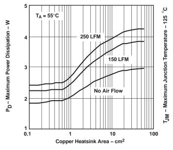
Figure 23. Maximum Power Dissipation vs Copper Heatsink Area
