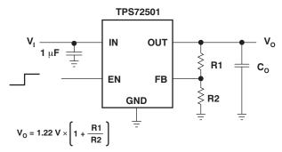
Figure 18. TPS72501 Adjustable Typical Application Diagram
