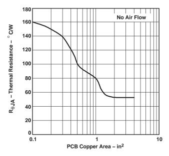
Figure 24. SOT223 Thermal Resistance vs PCB AREA
