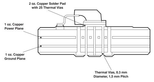
Figure 22. DDPAK Thermal Resistance
