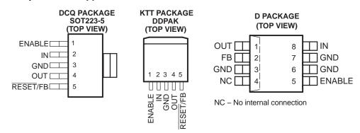
NOTE: TPS72501 replaces RESET with FB. Tab is GND for the DCK and KTT packages.
