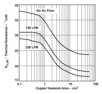
Figure 21. DDPAK Thermal Resistance vs Copper Heatsink Area
