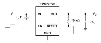
Figure 19. TPS72501 Fixed Output Typical Application Diagram
