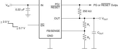
3.3 V 53.6 30.1 kΩ 3.6 V 61.9 30.1 kΩ NOTE: To reduce noise and prevent oscillation, R<sub>1</sub> and R<sub>2</sub> must be as close as possible to the
