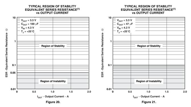
(1). Equivalent series resistance (ESR) refers to the total series resistance, including the ESR of the capacitor, any series resistance added externally, and PWB trace resistance to  $C_{OLIT}$ .
