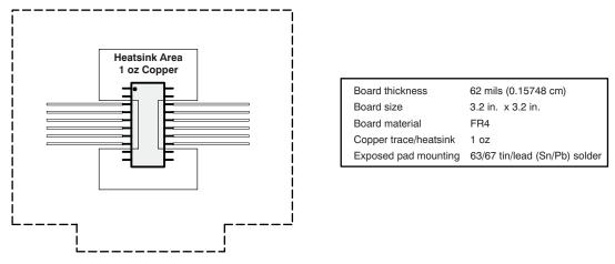
Figure 29. PWB Layout (Including Copper Heatsink Area) for Thermally-Enhanced PWP Package
